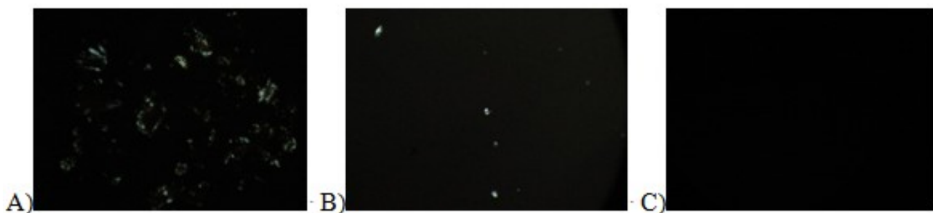
Fig. 1. Polarizing microscope images of ball-milled holocellulose (1.5 h) dissolved in [C 4 mim]Cl at 110 °C for 0 min (A), 30 min (B), and 170 min (C).
