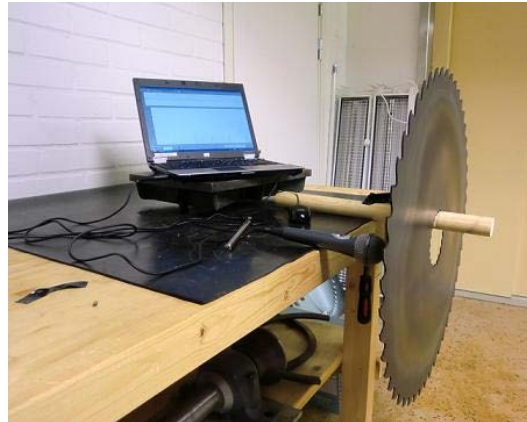
Fig. 4. Experimental installation for natural frequency measurement
