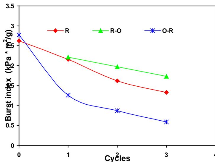
Fig. 4. Effects of R-O and O-R treatments on burst index
