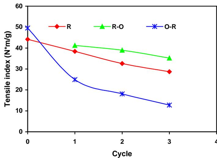
Fig. 3. Effects of R-O and O-R treatments on tensile index
