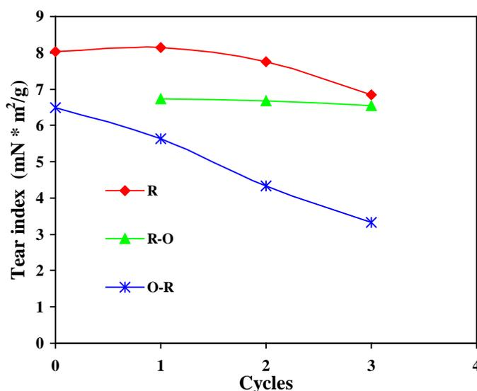
Fig. 5. Effects of R-O and O-R treatments on tear index
