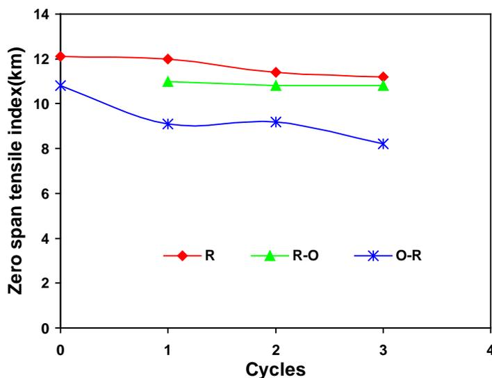
Fig. 6. Effects of R-O and O-R treatments on zero span tensile index
