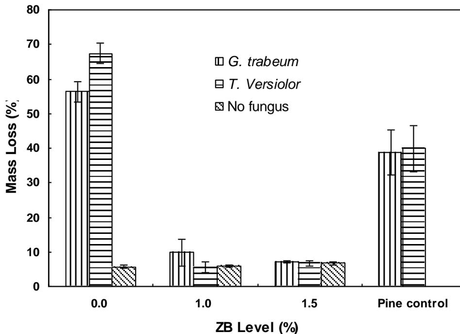
**Fig. 1.** Mass loss of untreated OSSB, pine solid wood, and ZB-treated OSSB exposed to the brown and white rot fungi in an AWPA E10 soil block test
