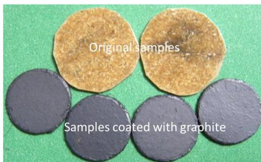
Fig. 2. Typical composite samples for thermal property analysis (Blend 5)
