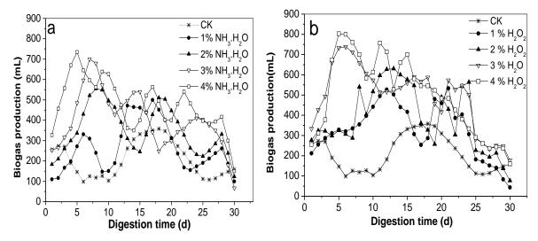
**Fig. 2.** Daily biogas production for each pretreatment. (a)  $NH_3 \cdot H_2O$  and (b)  $H_2O_2$  pretreatments CK: Rice straw without pretreatment
