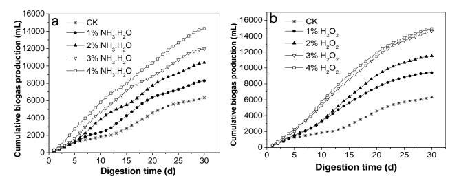
**Fig. 3.** Cumulative biogas production of each pretreatment. (a)  $NH_3 \cdot H_2O$  and (b)  $H_2O_2$  pretreatments. CK: Rice straw without pretreatment
