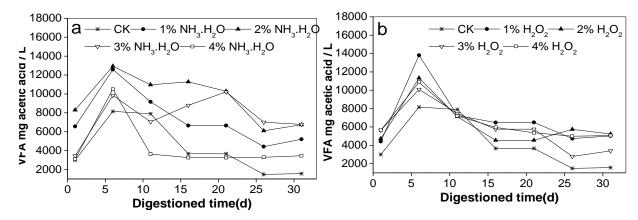
**Fig. 6.** VFA changes for each pretreatment. (a)  $NH_3 \cdot H_2O$  and (b)  $H_2O_2$  pretreatment. CK: Rice straw without pretreatment
