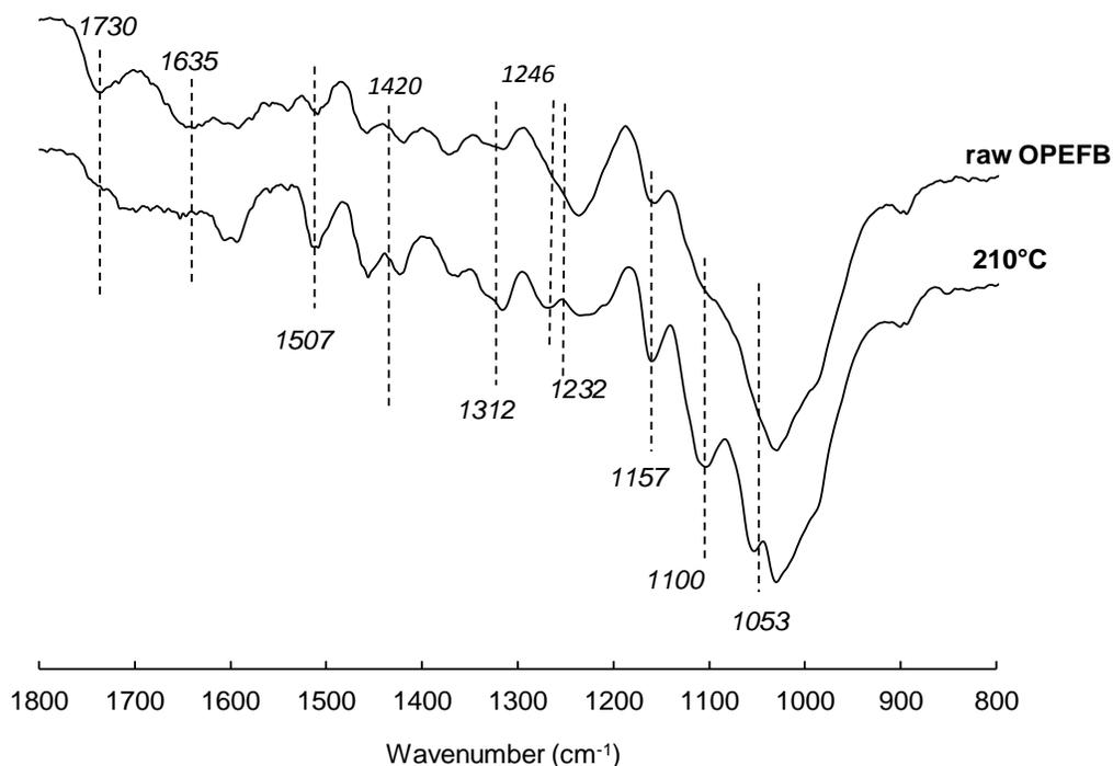
**Fig. 3.** FTIR spectra of raw and high-pressure steam treatment OPEFB for 210 °C
