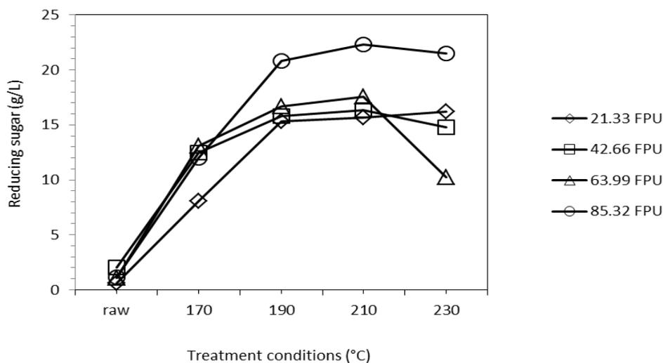
**Fig. 4.** Saccharification of treated OPEFB using different enzyme loading
