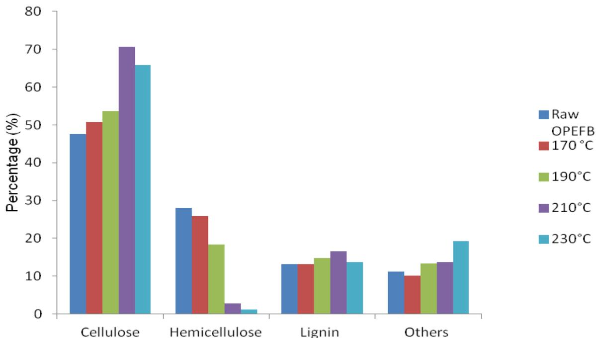
**Fig. 1.** Average compositions of elements in raw and high-pressure steam treated OPEFB at different temperatures
