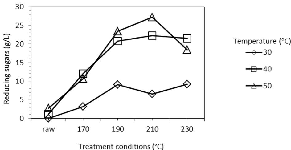
**Fig. 5.** Saccharification of raw and high-pressure steam treated OPEFB samples using different temperatures
