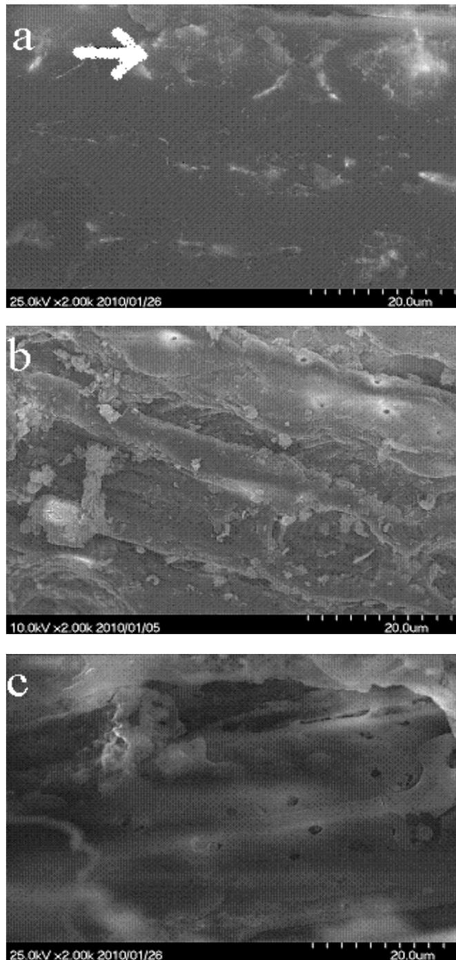
**Fig. 2.** SEM micrograph of raw OPEFB (a), high-pressure steam treated OPEFB at 210 °C (b), and at 230 °C (c). Arrow indicates silica bodies in the OPEFB strand
