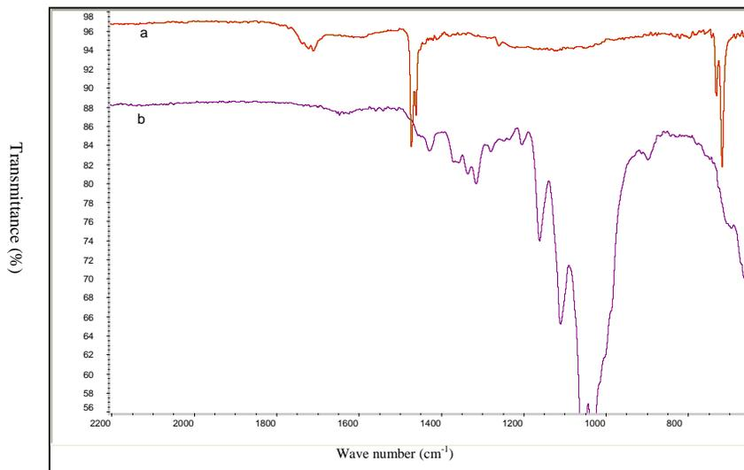
**Fig. 10.** FTIR spectra of control sample (a) and handsheet samples (b) from experiment carried out under optimum conditions
