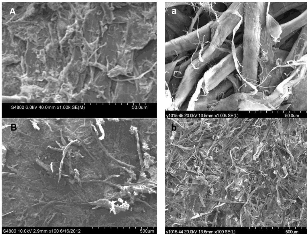
**Fig. 9.** SEM images of waste RMB paper at 1000 $\times$  (A) and 100 $\times$  (B) magnifications, and handsheets of fine pulp from waste RMB paper at 1000 $\times$  (a) and 100 $\times$  (b) magnifications
