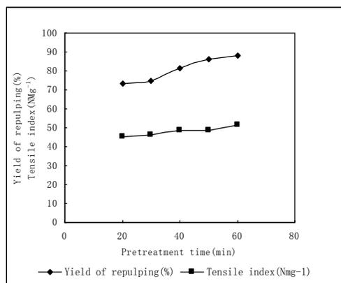
**Fig. 2.** Effect of pretreatment time on yield of repulping and tensile index (Pretreatment temperature 80 °C, waste paper consistency 10%, pretreatment time comprises of acid and alkali pretreatment)
