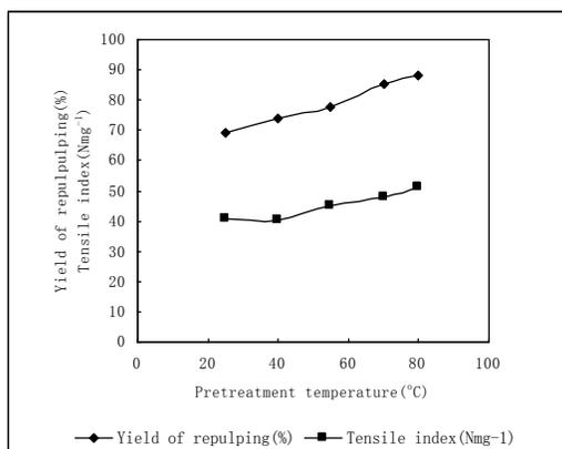
**Fig. 1.** Effect of pretreatment temperature on repulping yield and tensile index (Pretreatment time 60 min and waste paper consistency 10%)
