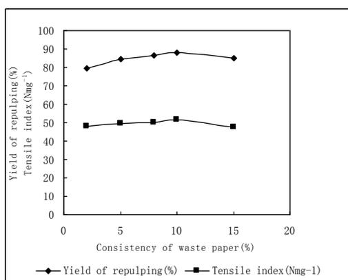
**Fig. 3.** Effect of pretreatment concentration on yield of repulping and tensile index (Pretreatment time 60 min and pretreatment temperature 80 °C)
