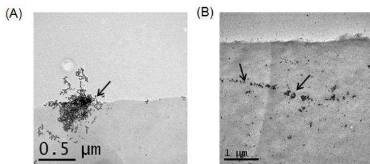
**Fig. 3.** Representative TEM micrographs of *M. floridulus* stem tissues with absorbed gold nanoparticles at a magnification of 10,000 $\times$  (A) and 6,000 $\times$  (B), respectively. Gold nanoparticles shown as black dots are indicated by arrows.
