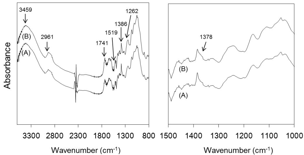
**Fig. 5.** Representative FT-IR spectra of *M. floridulus* stems with or without gold nanoparticles. The frequency region between 1000 and 1500  $\text{cm}^{-1}$  was expanded in the right-hand plot. (A) *M. floridulus* stems; (B) *M. floridulus* stems in the presence of gold nanoparticles.
