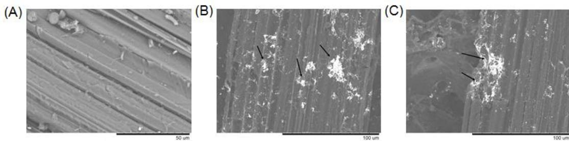
**Fig. 4.** Representative SEM images of *M. floridulus* stems with or without gold nanoparticles at a magnification of (A) 1,000 $\times$ ; (B) 1,500 $\times$ ; (C) 1,500 $\times$ . Gold nanoparticles appeared as white spots were indicated by arrows.
