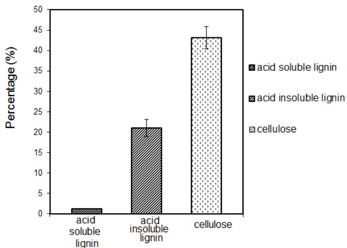
**Fig. 1.** Lignin, cellulose, and ash contents of *M. floridulus* stems
