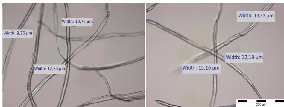
**Fig. 2.** Optical images of the bleached eucalyptus pulp fibres before sonication treatments
