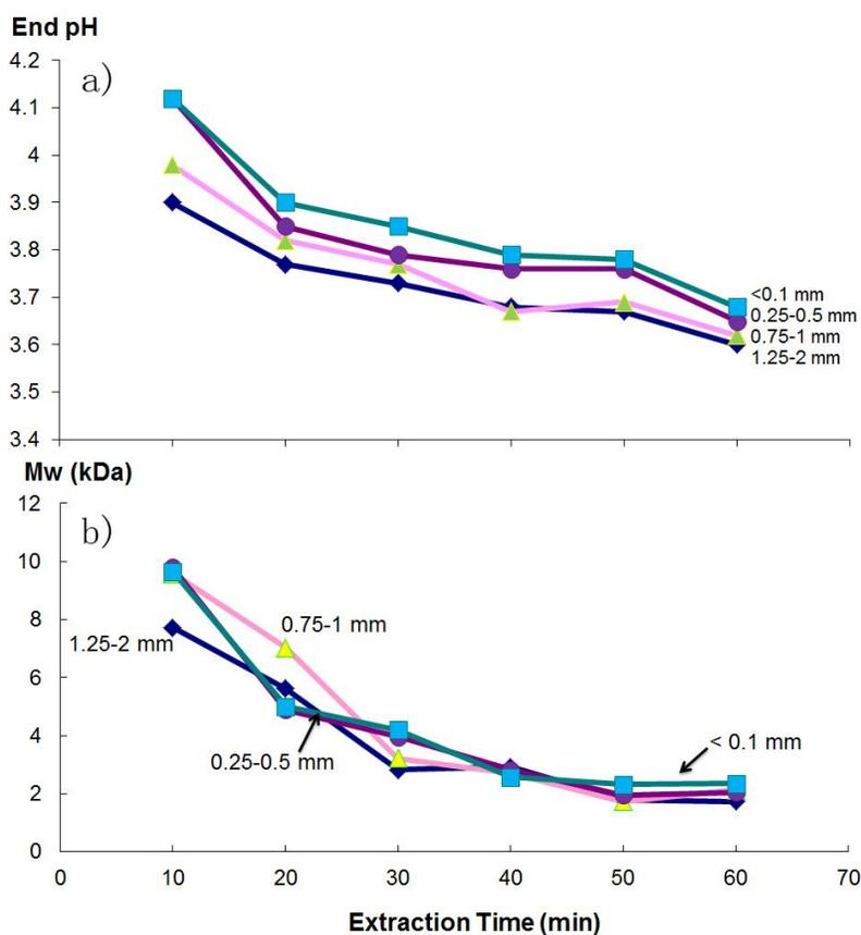
**Fig. 3.** a) End-pH of the water extract solutions, measured at room temperature, and b) Average  $M_w$  of extracted hemicelluloses.
