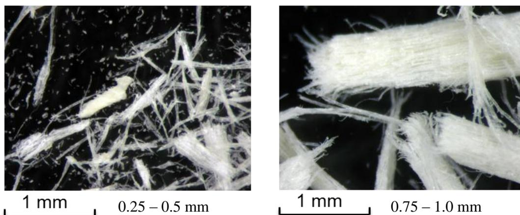
**Fig. 1.** Microscopy images of two ground spruce wood fractions
