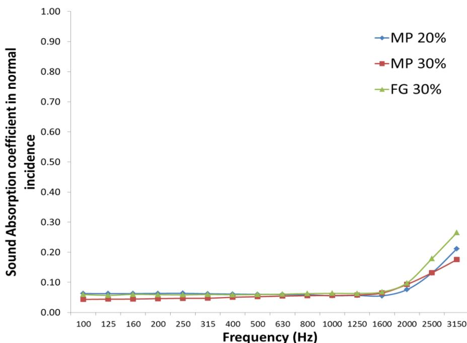
Fig. 3. Sound absorption coefficient vs. frequency of some studied composite materials
