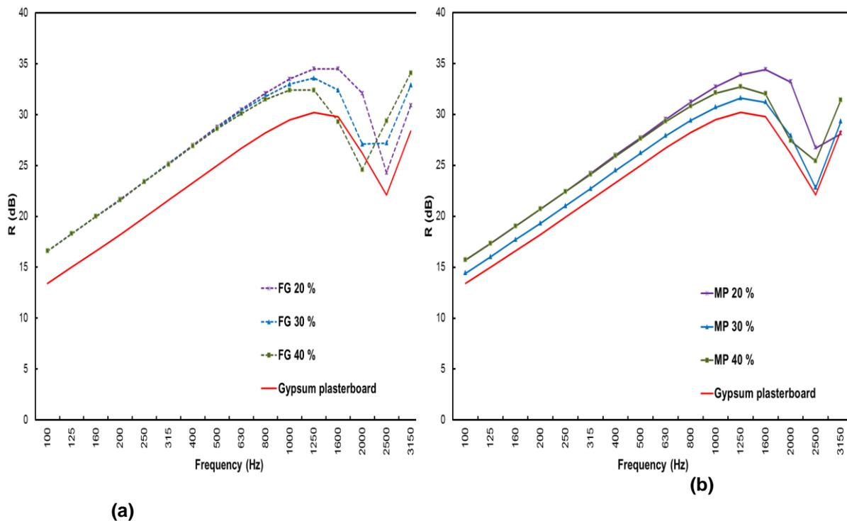
**Fig. 4.** Prediction of the acoustic isolation for MP and FG composites considered as an impermeable single-layer: (a) fiberglass, (b) mechanical pulp fibers. Comparison with gypsum plasterboard
