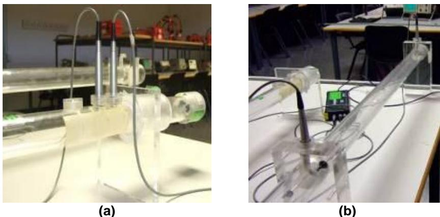
**Fig. 2.** Experimental equipments for measurement of (a) sound absorption coefficient (UNE EN ISO 10534-2:2004), and (b) the specific resistance to flow (Ingard & Dear method)
