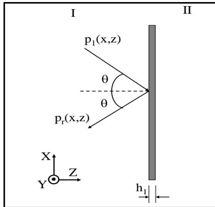
**Fig. 1:** Thin and impermeable plate separating two spaces
