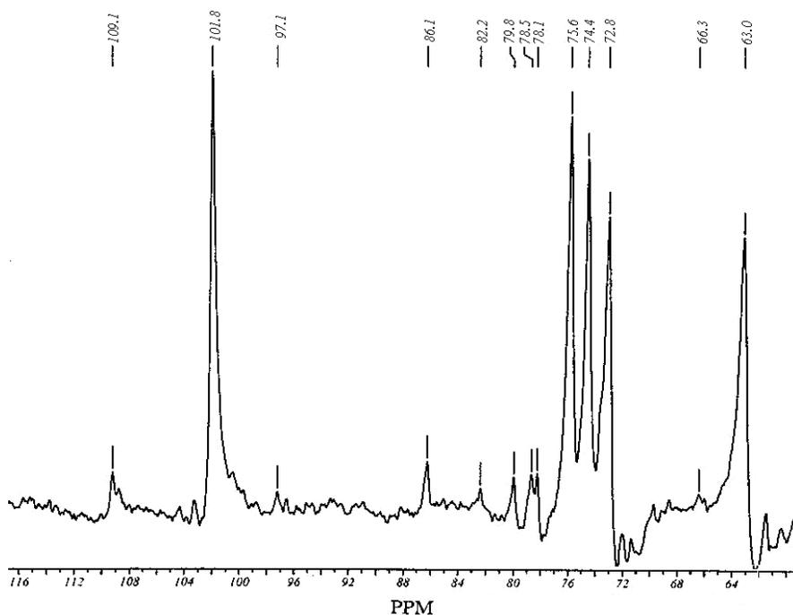
Fig. 5.  $^{13}\text{C}$ -NMR spectrum of hemicellulosic fraction H<sub>4</sub>
