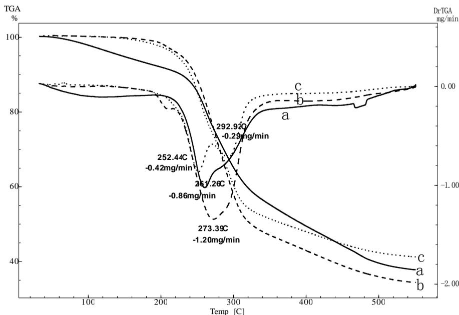
**Fig. 6.** TGA/DTG of hemicellulosic fractions H<sub>2</sub> (curve a), H<sub>4</sub> (curve b), and H<sub>5</sub> (curve c)
