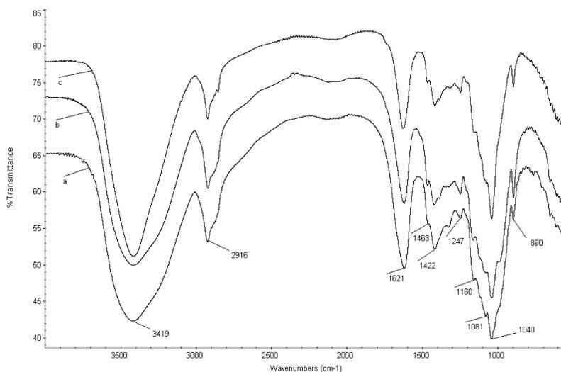
**Fig. 3.** Spectra of hemicellulosic fractions  $H_4$  (spectrum *a*),  $H_5$  (spectrum *b*), and  $H_6$  (spectrum *c*)
