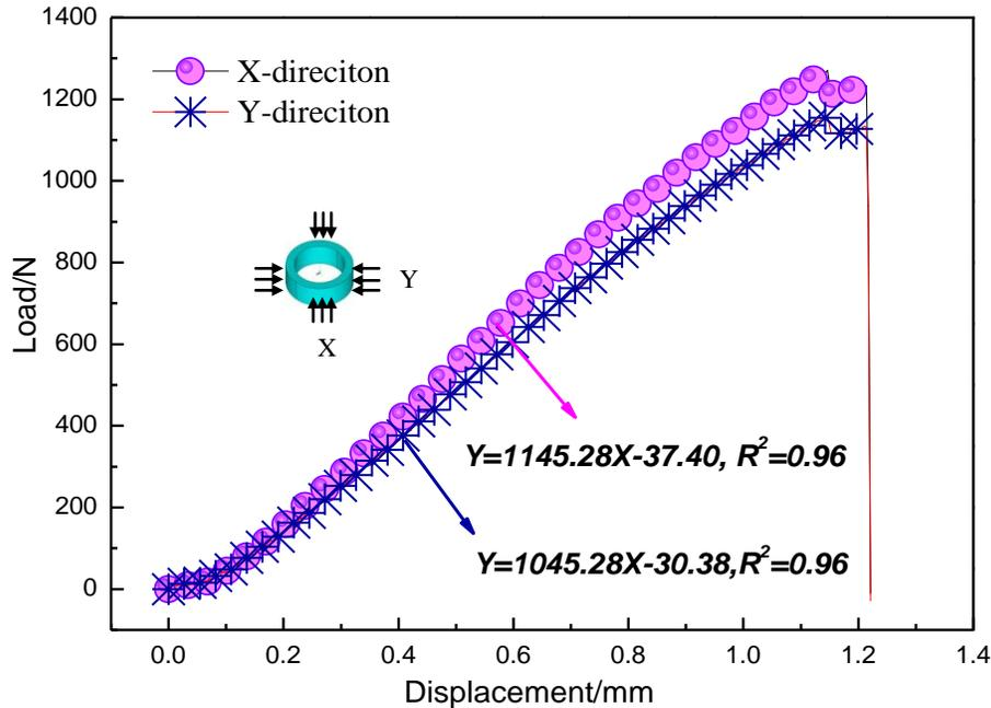
Fig. 2. Typical load displacement curves of bamboo ring under biaxial loading
