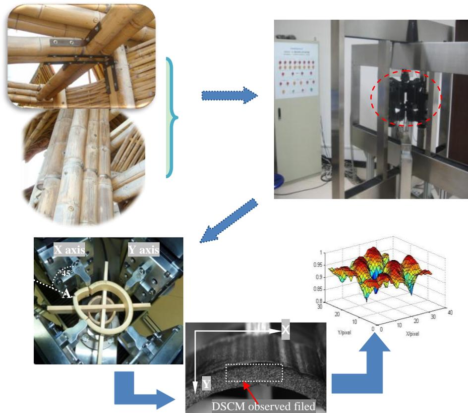
**Fig. 1.** Bamboo structure, 3D composite material analysis system, and visual field of specimen by DSCM. (Arrow represents the positive direction of strain-fields chosen for calculation.)
