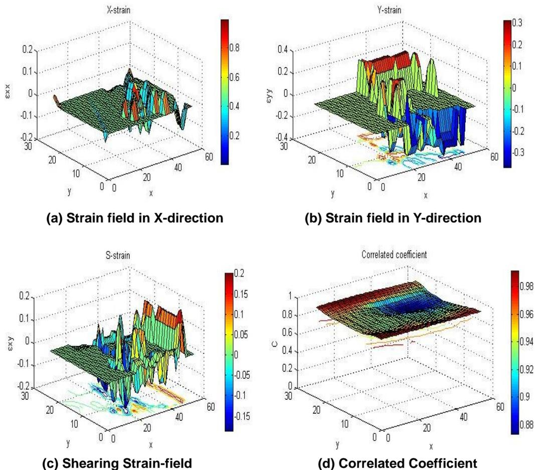
**Fig. 6.** The information of strain field under biaxial compression load between 0~300 N
