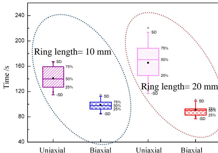
**Fig. 4.** The effect of loading methods on the breaking time of bamboo ring
