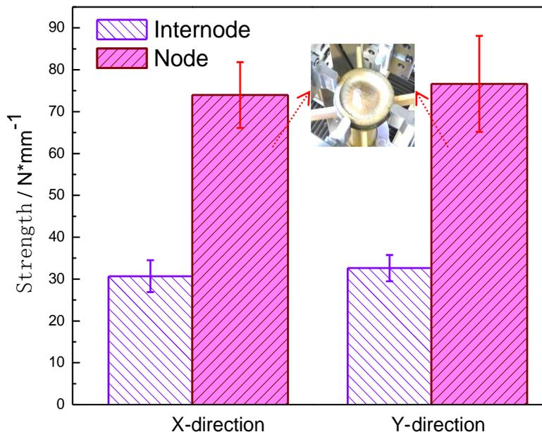
**Fig. 5.** The effect of node on the radial-circumferential strength under biaxial loading
