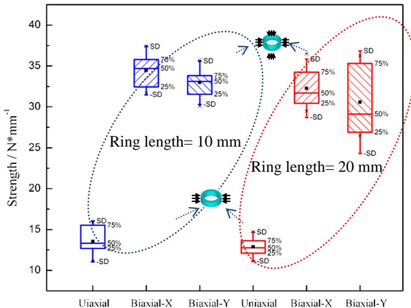
Fig. 3. The effect of loading methods on the compression strength of bamboo ring
