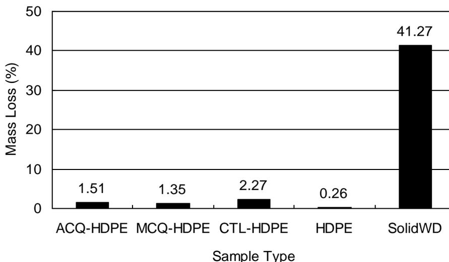
Fig. 3. The mass loss of different composite samples after decay test
