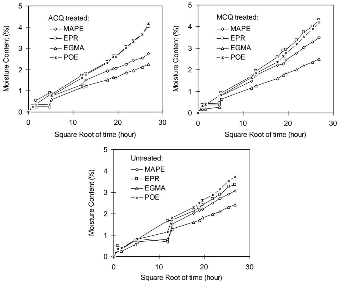
**Fig. 2.** Moisture absorption vs. time for treated and untreated wood-filled HDPE composites with different coupling agents
