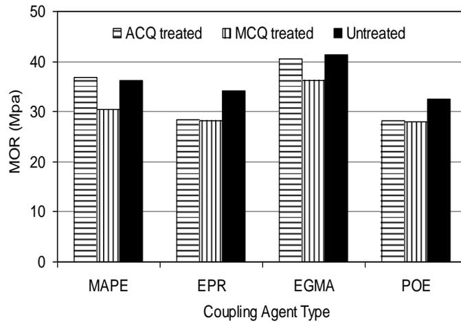
**Fig. 1.** Modulus of rupture (MOR) for treated and untreated wood-filled HDPE composites
