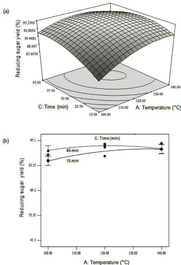
**Fig. 1.** (a) Three-dimensional response surface plot of the effect of pretreatment temperature and duration on the RS yield at 0.5 M NaOH; (b) Interaction plot between pretreatment temperature and duration on the RS yield at 0.5 M NaOH
