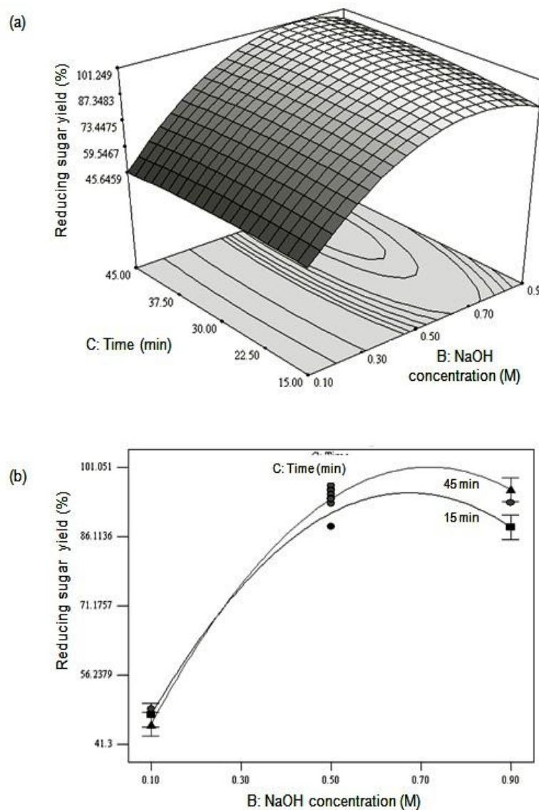
**Fig. 2.** (a) Three-dimensional response surface plot of the effect of pretreatment duration and NaOH concentration on the RS yield at 120°C (b) Interaction plot between pretreatment duration and NaOH concentration on the RS yield at 120°C
