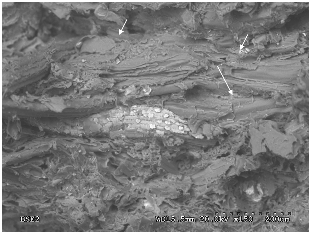
Fig. 5. SEM micrographs: (A) fractured surface of particleboard D1 manufactured with 5% of potato starch and two hot-pressings; (B) fractured surface of panel D3 made with 10% of potato starch and three hot-pressings
