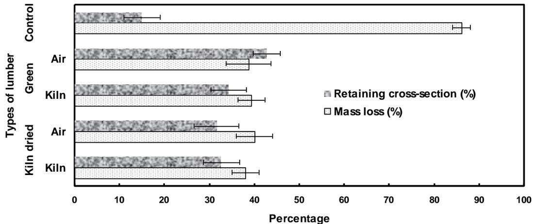
Fig. 6. Mass loss (%) and cross-section retention (%) for different lumber types after a fire test
