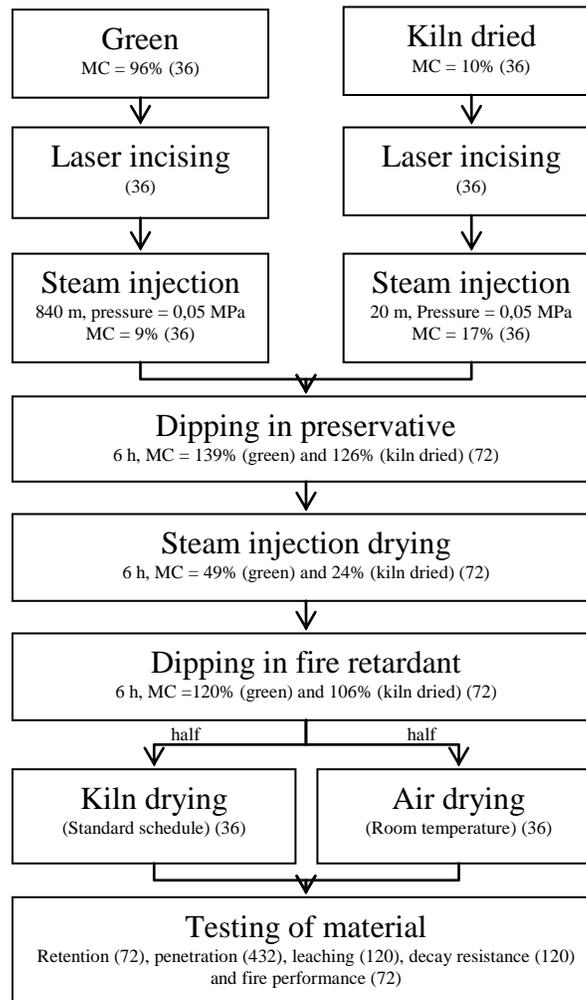
**Fig. 2.** Flow diagram of the experimental process. The data in parentheses are the numbers of samples.
