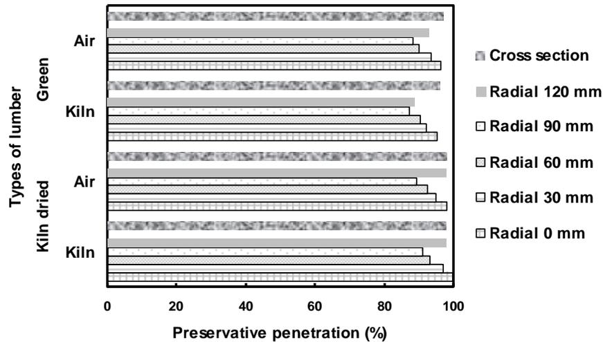
Fig. 4. Cross sectional and radial surface preservative penetration area for different types of lumber
