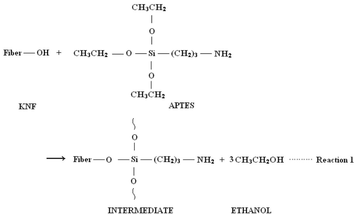
**Fig. 1.** Proposed possible interactions scheme between KNF and 3-aminopropyltriethoxysilane (APTES) coupling agent
