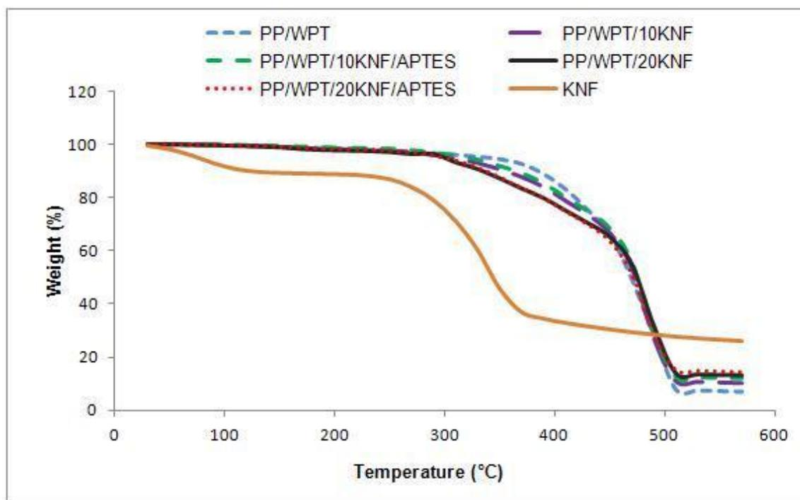
**Fig. 3.** TGA curves of KNF and PP/WPT/KNF composites with and without 3-aminopropyltriethoxysilane (APTES)
