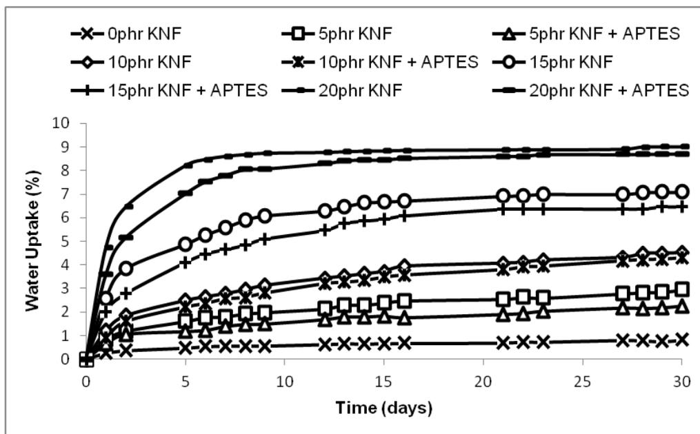
**Fig. 2.** Water uptake of PP/WPT/KNF (70/30) composites with and without 3-aminopropyltriethoxysilane (APTES)
