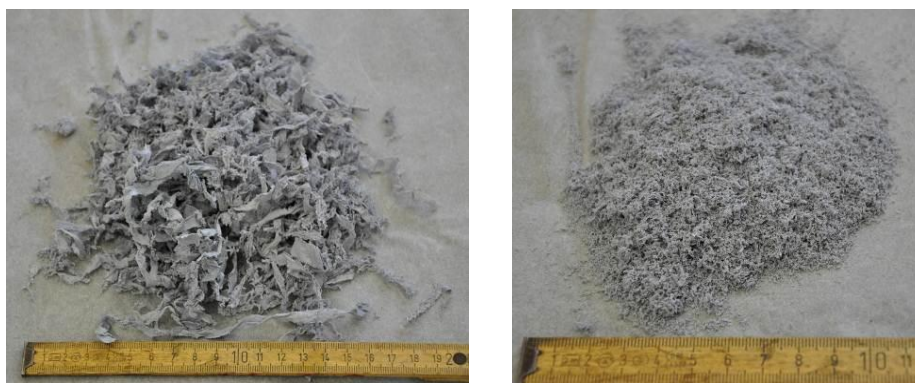
Fig. 1. Wet-blue leather shavings before (left) and after sieving (right)
