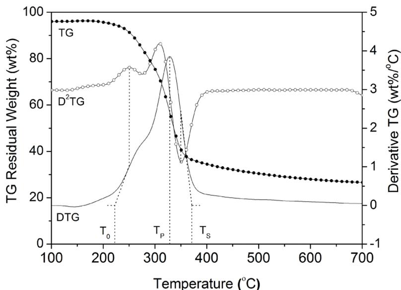
**Fig. 2.** Determination of decomposition characteristic parameters of heat-treated fibers using 150°C heat-treated BFs as an example at a heating rate of 5°C/min
