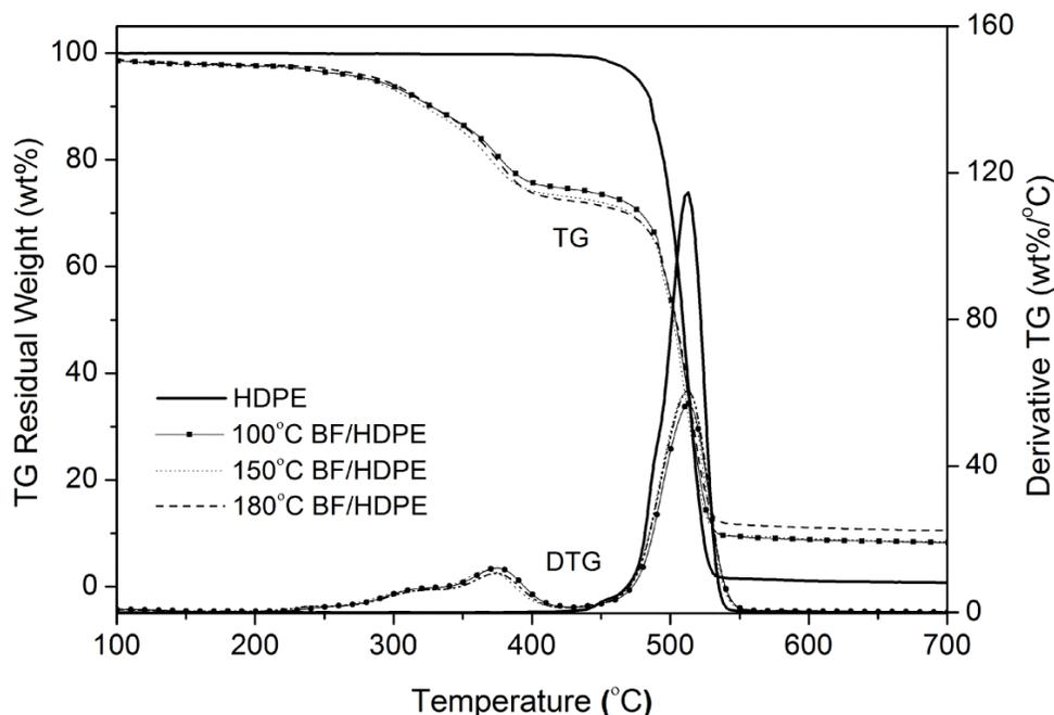
**Fig. 5.** Thermo-gravimetric decomposition process of heat-treated BFs and HDPE blends at the heating rate of 40°C/min
