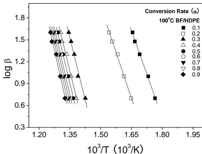
Fig. 7. Typical iso-conversional plot of Flynn-Wall-Ozawa method for bamboo fiber/HDPE blends
