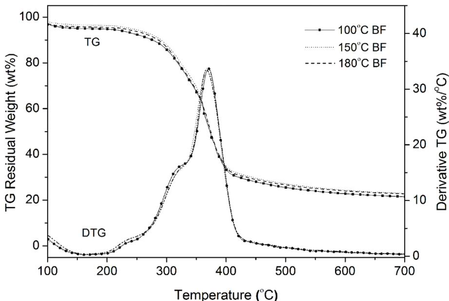
**Fig. 1.** Thermo-gravimetric decomposition process of heat-treated BFs at the heating rate of 40°C/min
