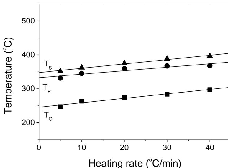
**Fig. 3.** Determination of decomposition characteristic parameters (*i.e.*, onset, peak, and shift temperatures) of heat-treated fibers using 100°C heat-treated BFs as an example
