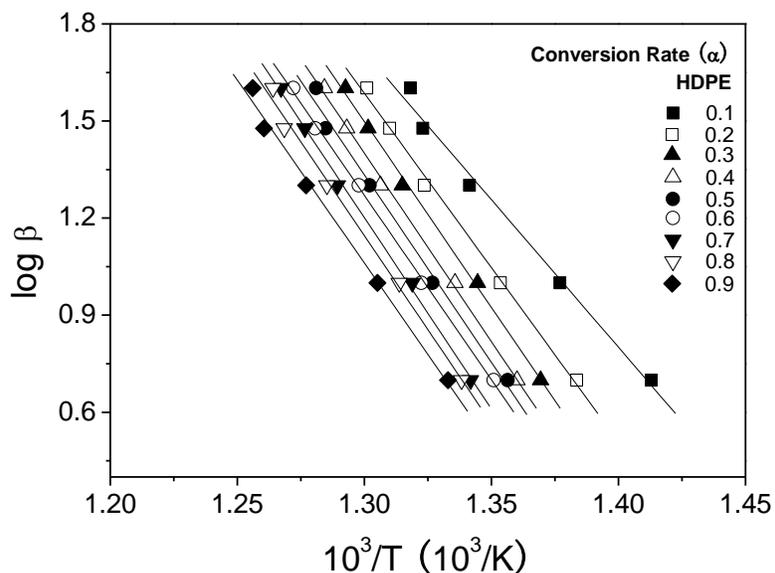
Fig. 6. Typical iso-conversional plot of Flynn-Wall-Ozawa method for pure HDPE
