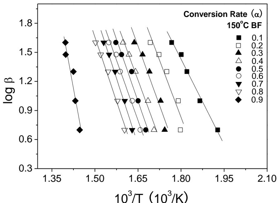
Fig. 4. Typical iso-conversional plot of the Flynn-Wall-Ozawa method
