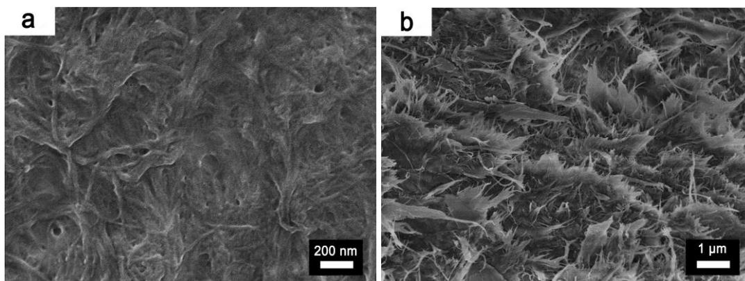
Fig. 4. FE-SEM image of (a) undamaged surface of nanopaper and (b) nanopaper surface pierced and torn by a needle
