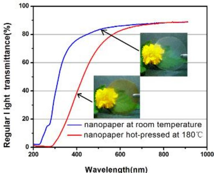
**Fig. 6.** Regular light transmittances of nanopaper at room temperature and nanopaper that was hot-pressed at 180 °C
