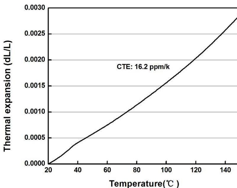
**Fig. 7.** Coefficient of thermal expansion (CTE) of the nanopaper made with CNFs from waste corrugated paper
