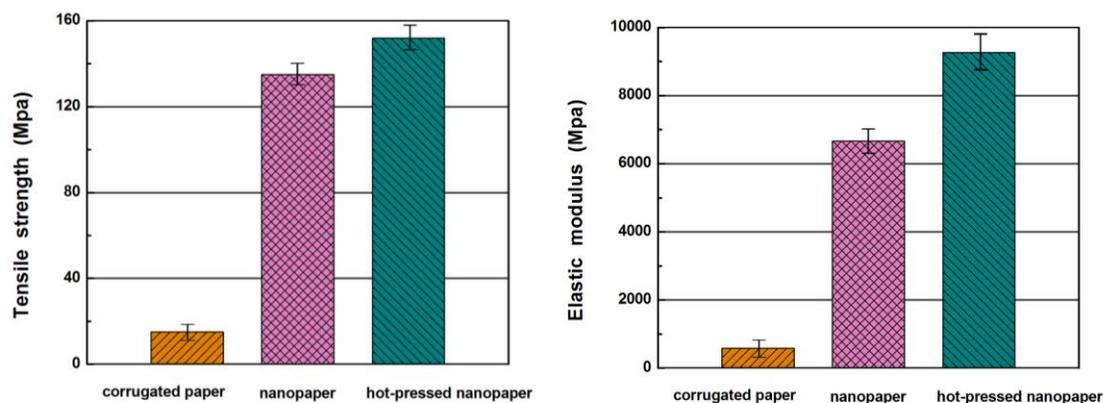
**Fig. 5.** Tensile properties of untreated waste corrugated paper, nanopaper at room temperature, and nanopaper hot-pressed at 180 °C
