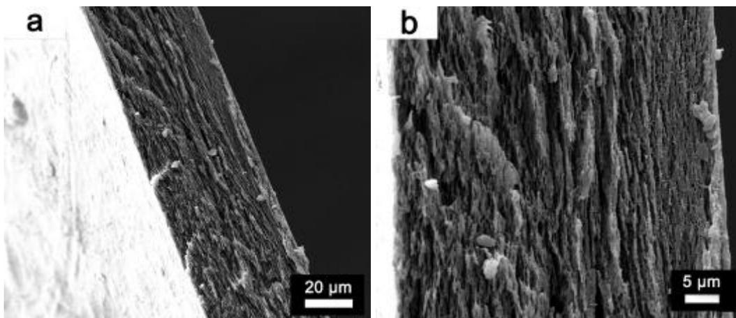
Fig. 3. SEM micrographs of the fracture surface of the cellulose nanopaper
