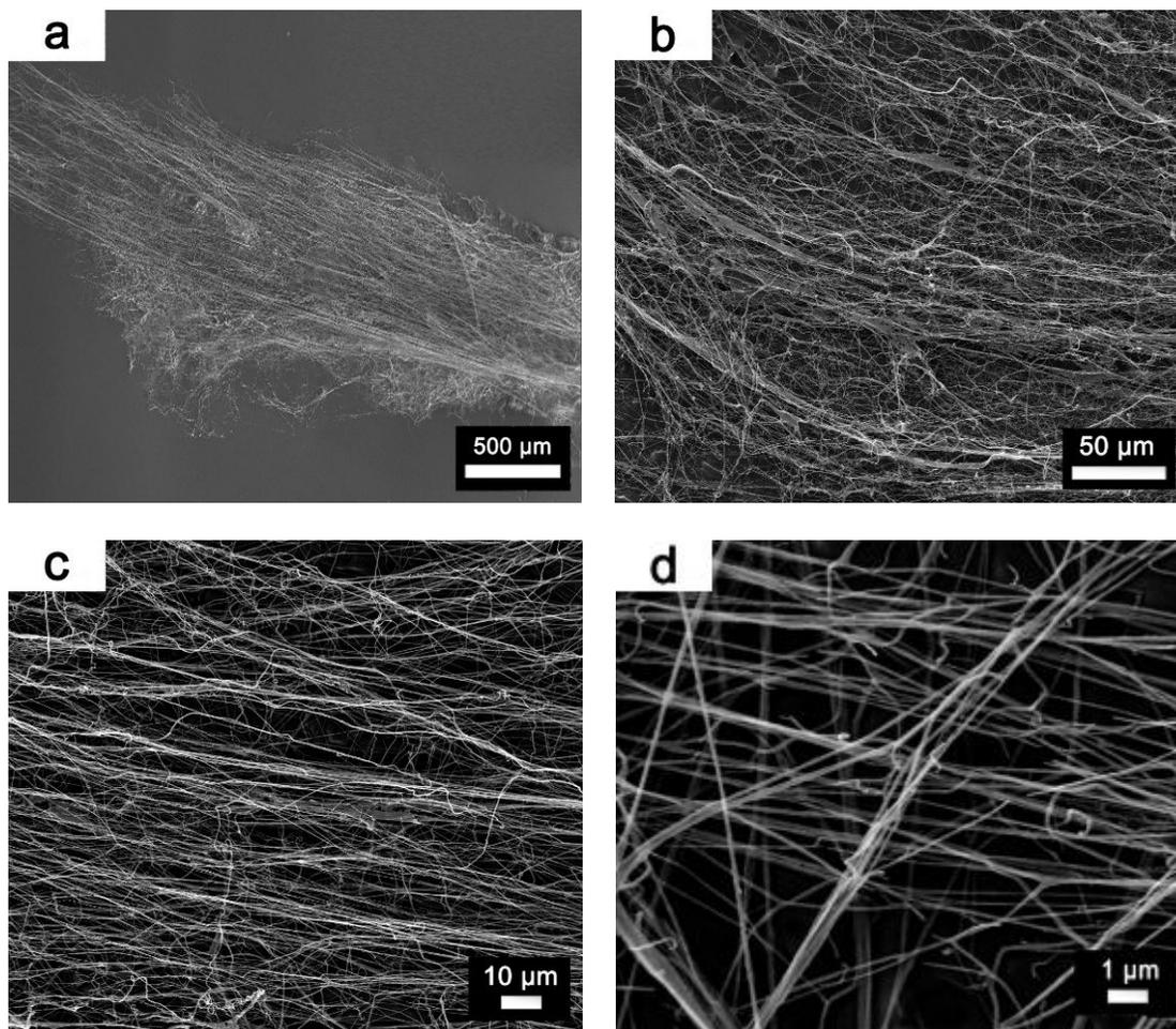
**Fig. 2.** SEM observation of ultralong CNFs assembled from slender cellulose nanofibrils
