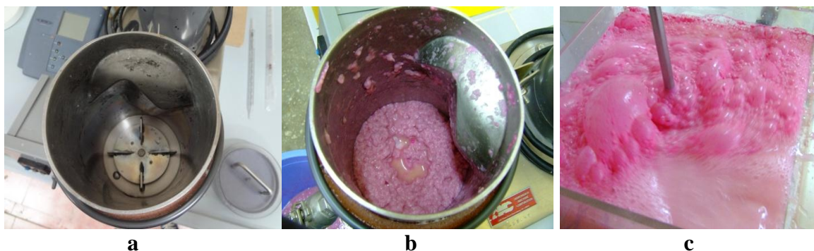
Fig. 1. Micro-Maelstrom pulper rotor (a), pulping process (b), and flotation process (c)
