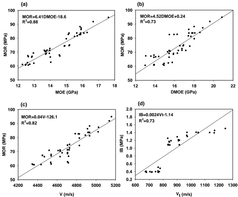
**Fig. 3.** Relationship between different properties of the OSBs: (a) MOR and MOE, (b) MOR and DMOE, (c) MOR and  $V$ , and (d) IBs and  $V_t$
