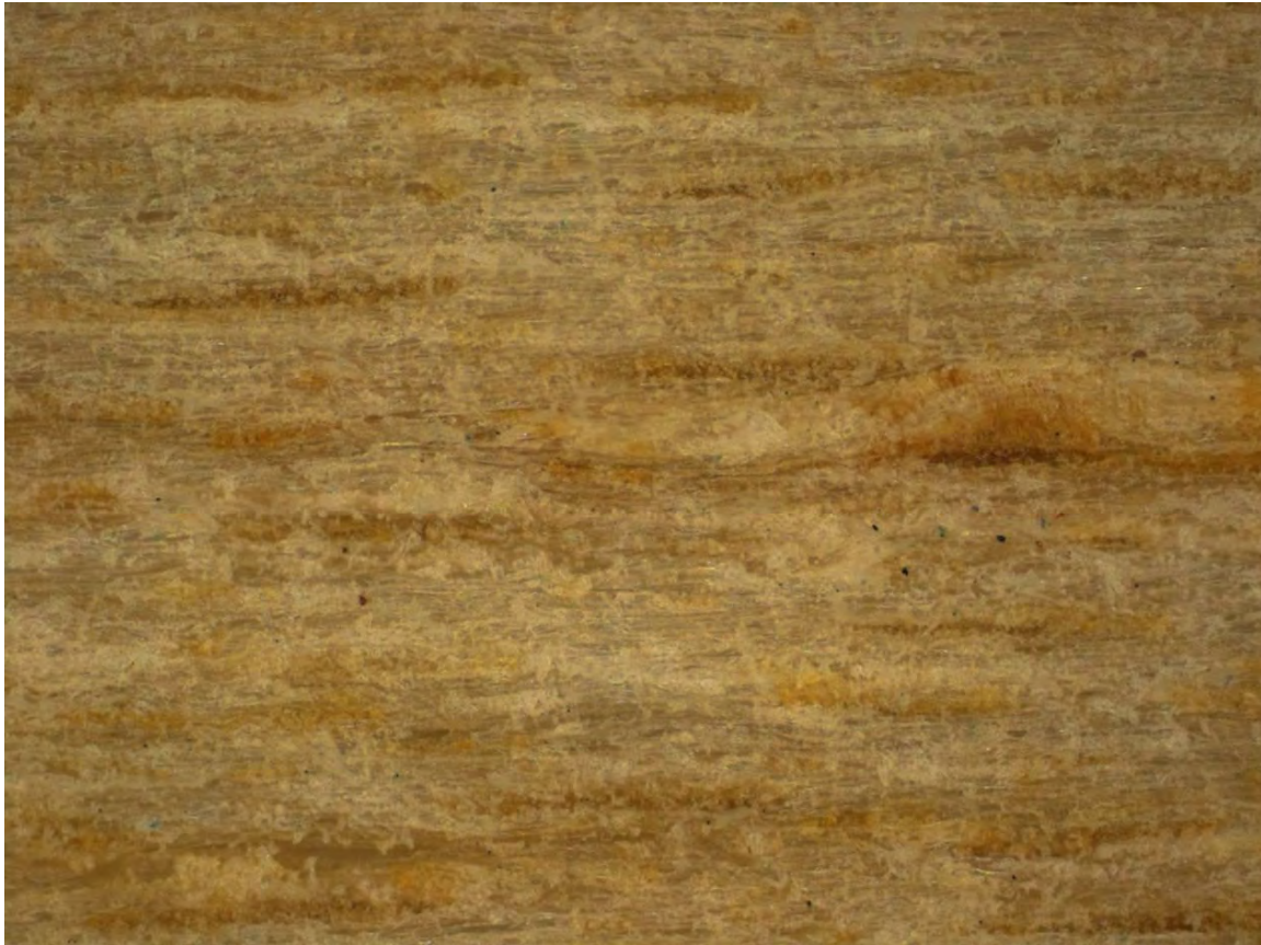
Fig. 4. Surface of a peeled veneer without finishing products and its longitudinal parenchyma
