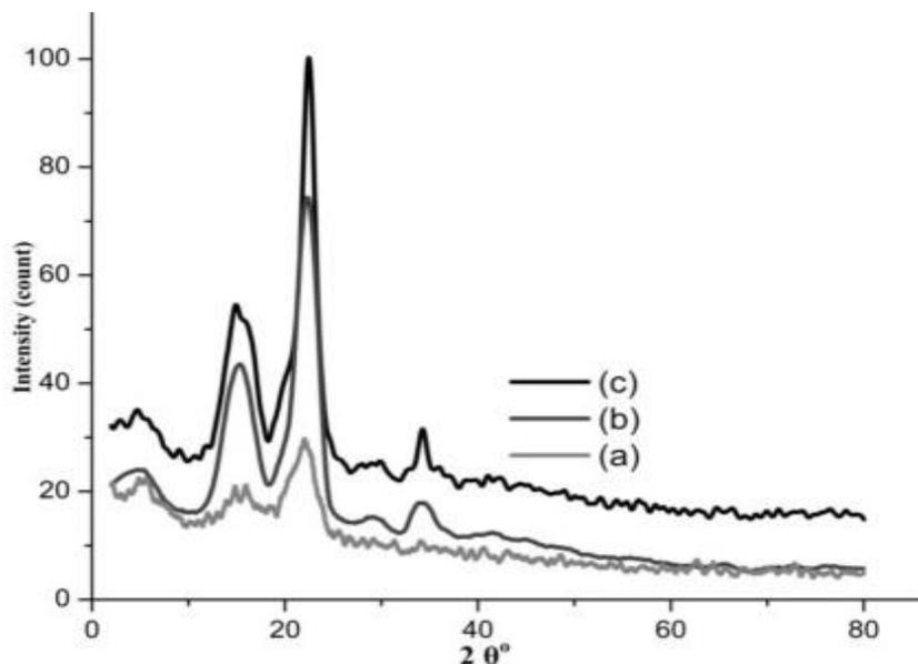
**Fig. 4.** X-ray diffractogram of (a) raw OPEFB, (b) extracted OPEFB-cellulose, (c) commercial MCC
