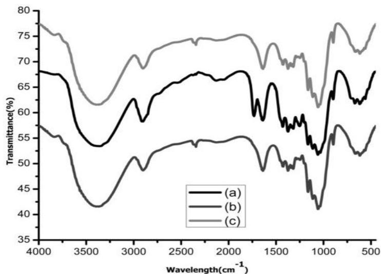
**Fig. 3.** FTIR of (a) raw OPEFB, (b) extracted OPEFB-cellulose, (c) commercial MCC
