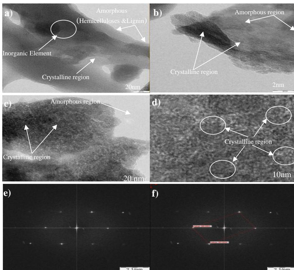
**Fig. 2.** TEM micrograph of (a & b) raw OPEFB; (c & d) extracted cellulose; (e) the diffraction pattern; (f) the monoclinic pattern and its measurement
