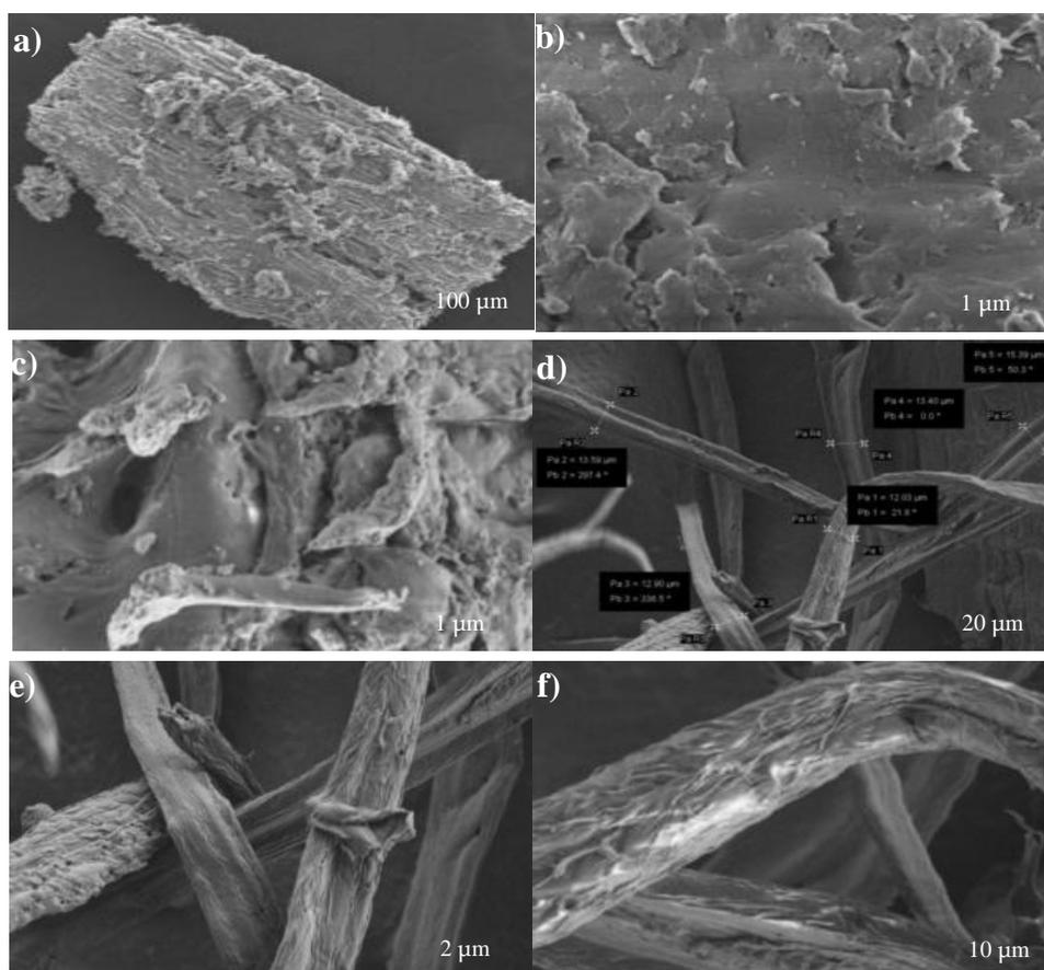
**Fig. 1.** FESEM micrographs of (a-c) raw OPEFB; (d-f) extracted OPEFB-cellulose
