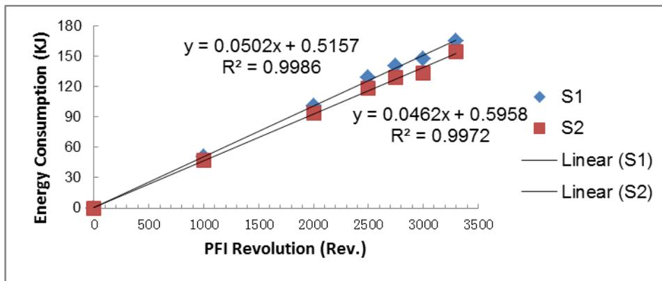
**Fig. 1.** The linear relationship of energy consumption and PFI refining revolutions
