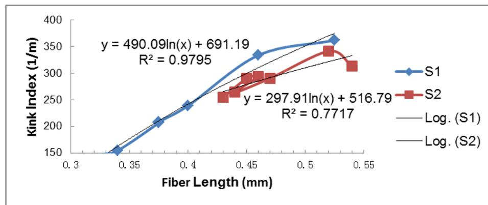
Fig. 4. The logarithmic relationship of kink index and fiber length
