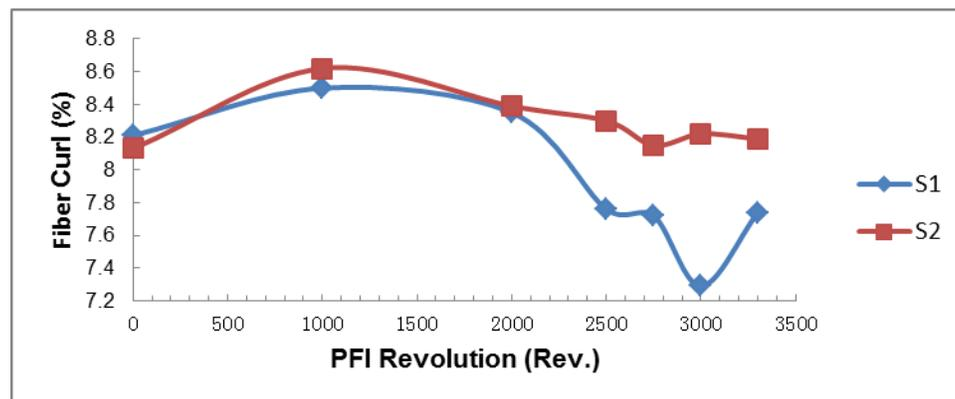
Fig. 5. The irregular relationship of fiber curl and PFI refining revolutions
