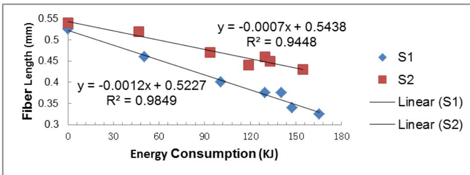
**Fig. 2.** The linear relationship of fiber length and energy consumption
