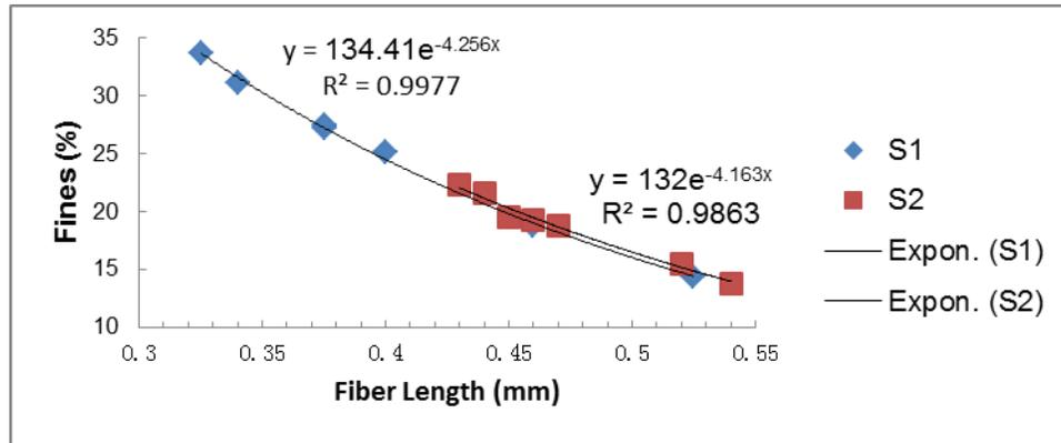
Fig. 3. The exponential relationship of fines and fiber length
