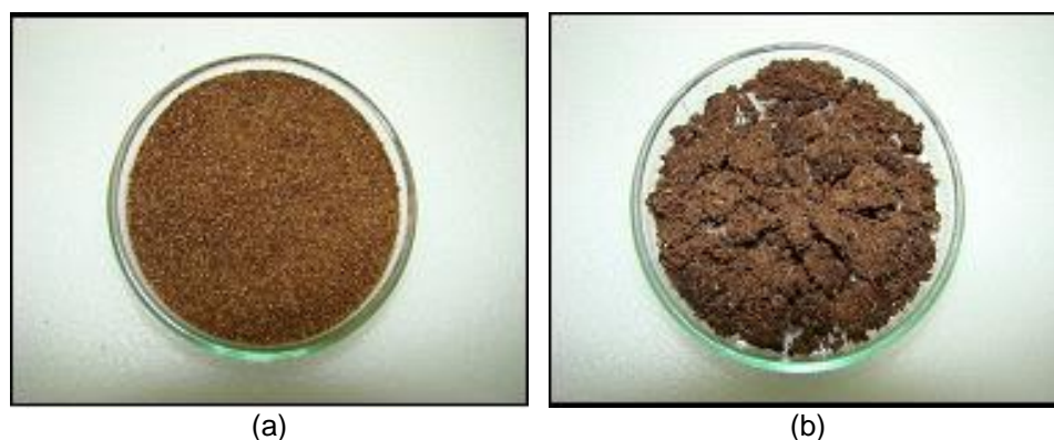
Fig. 1. (a) Banana fibers (BF) and (b) washed banana fibers (WBF)
