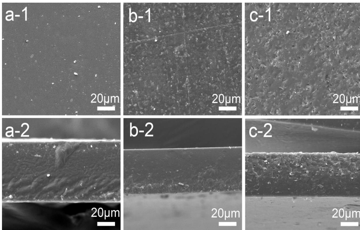
**Fig. 2.** SEM micrographs of the membranes: membrane L-0 ( $\times 1000$ ; a-1 surface, a-2 cross section); blend membrane L-2 ( $\times 1000$ ; b-1 surface, b-2 cross section); blend membrane L-5 ( $\times 1000$ ; c-1 surface, c-2 cross section)
