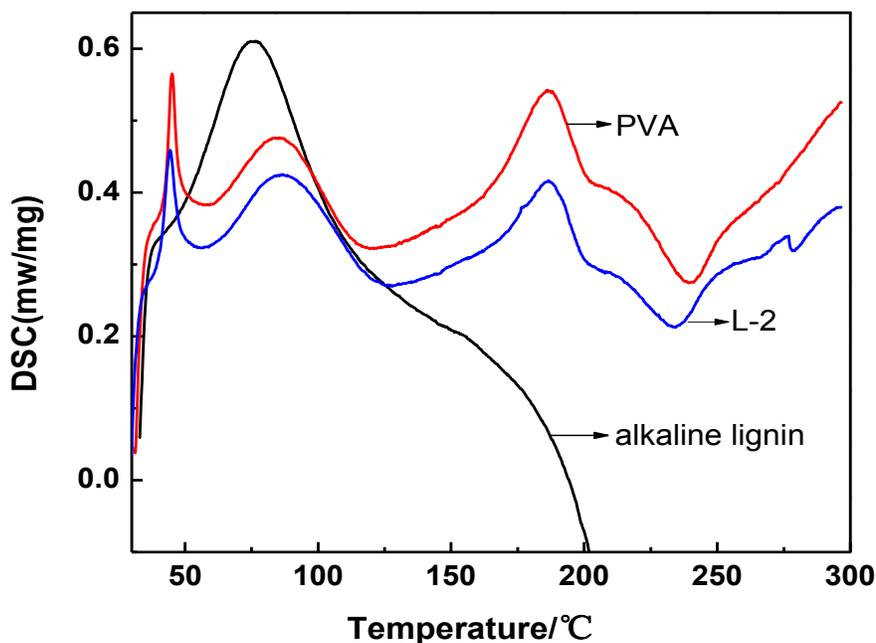
**Fig. 4.** DSC thermograms of alkaline lignin, PVA, and blend membrane L-2
