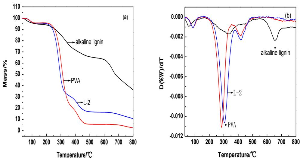
Fig. 3. TG and DTG diagram of alkaline lignin, PVA and blend membrane L-2: (a) TG; (b) DTG
