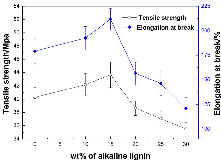
Fig. 1. Effect of quantity of alkaline lignin on tensile strength
