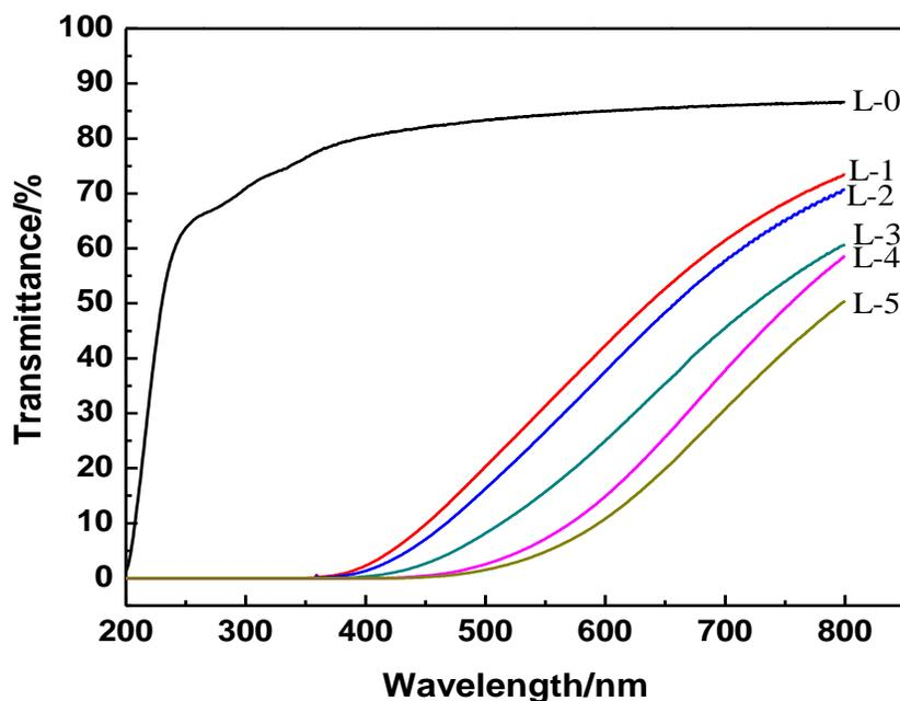
Fig. 5. UV-visible spectra of the membranes
