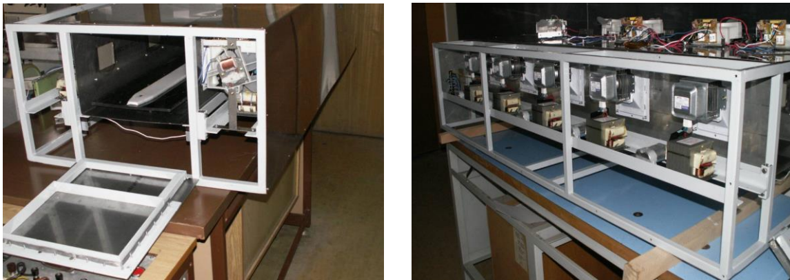
Fig. 1. Microwave plasticizing device, an overview ( left ) and placement of cavity magnetrons ( right )
