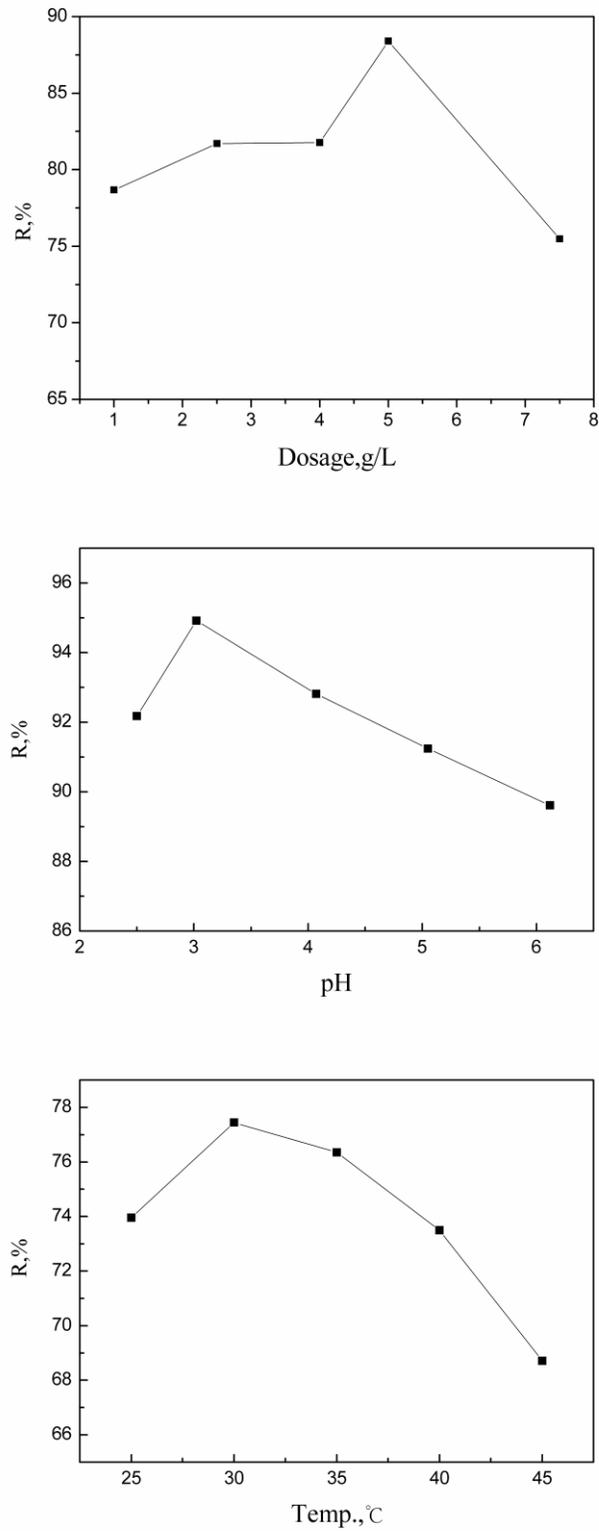
**Fig. 5.** Effect of different conditions on the removal of Acid black ATT
