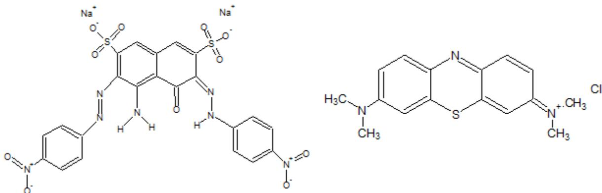
**Fig. 4.** Molecular structure of acid black (left) and methylene blue (right)
