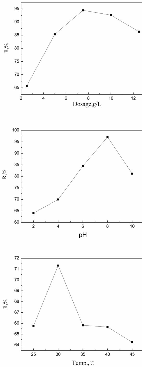
**Fig. 6.** Effect of different conditions on the removal of methylene blue
