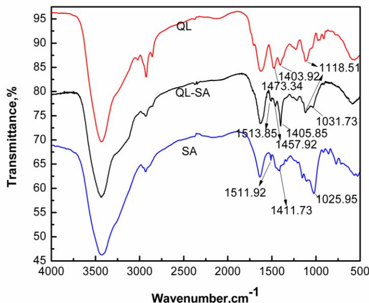
Fig. 2. FT-IR spectrum of QL (top), QL-SA (middle), and SA (bottom)
