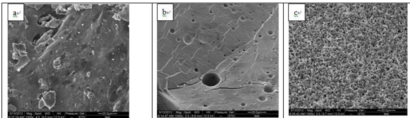
**Fig. 3.** SEM photographs of SA(a, 1000x), QL(b, 1000x), and QL-SA(c, 1000x)
