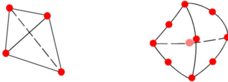
**Fig. 3.** Network of finite elements - linear tetrahedral element (left) and parabolic tetrahedral element (right)
