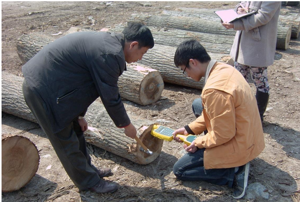
Fig. 1. Resonance-based log acoustic test with Director HM 200™
