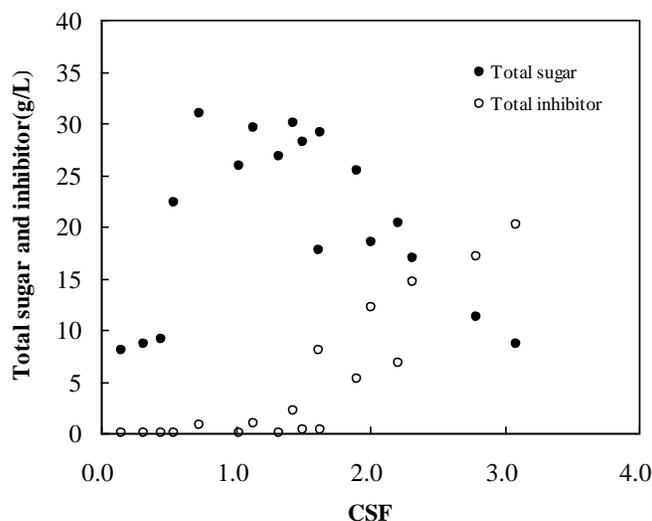
Fig. 4. Concentration of total sugar and inhibitors as a function of combined severity factor (CSF)
