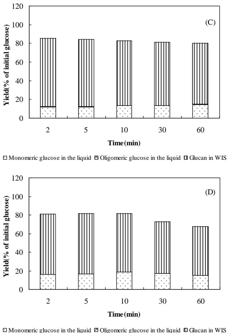
**Fig. 3(c-d).** Yield of glucose in liquids and water-insoluble solids (WISs) from the pretreatments with 0.60%  $\text{HNO}_3$  at (A) 80°C; (B) 120°C; (C) 150°C; and (D) 180°C
