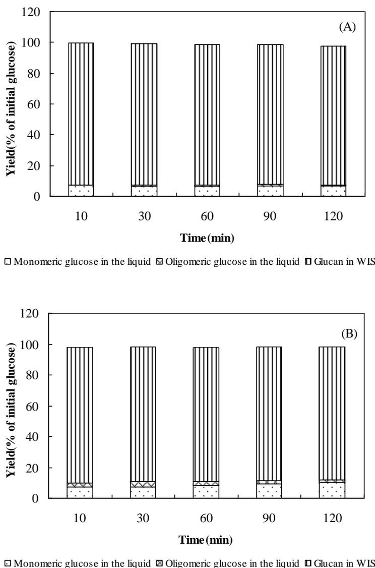
**Fig. 3(a-b).** Yield of glucose in liquids and water-insoluble solids (WISs) from the pretreatments with 0.60% HNO<sub>3</sub> at (A) 80°C; (B) 120°C; (C) 150°C; and (D) 180°C
