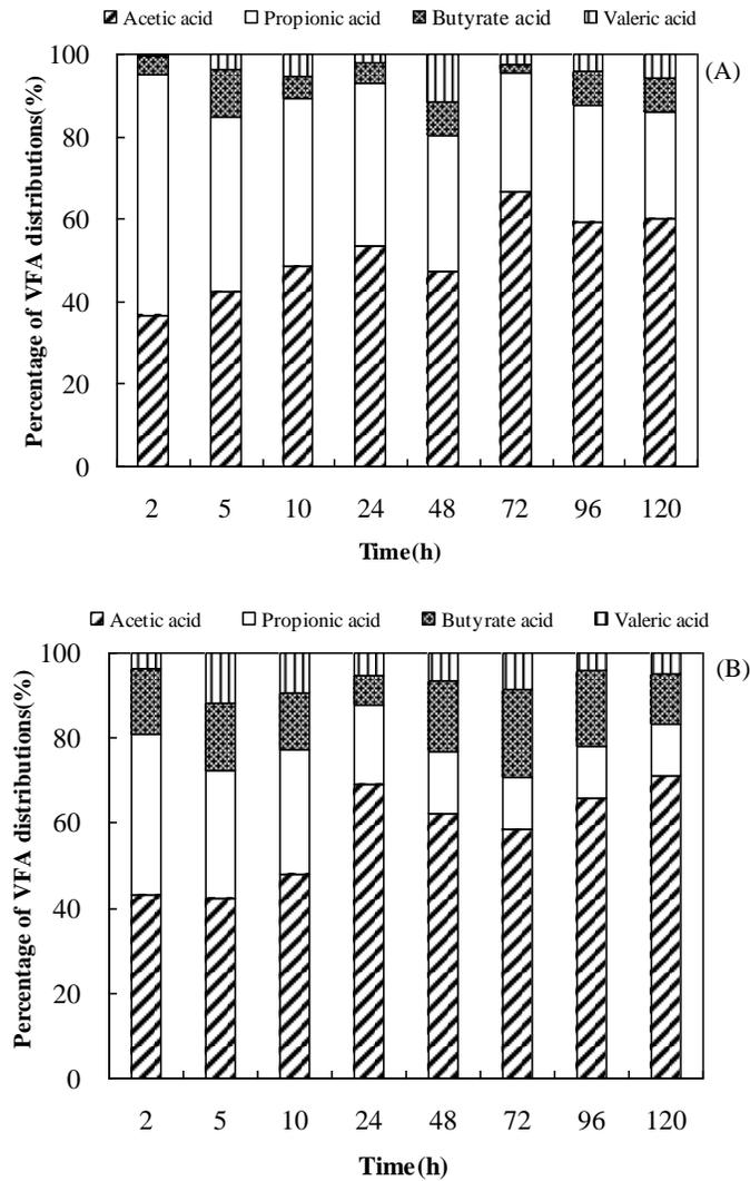
**Fig. 6.** Distribution of VFAs at the final state of anaerobic acidogenic fermentation of (A) raw corn stover and (B) hydrolysate
