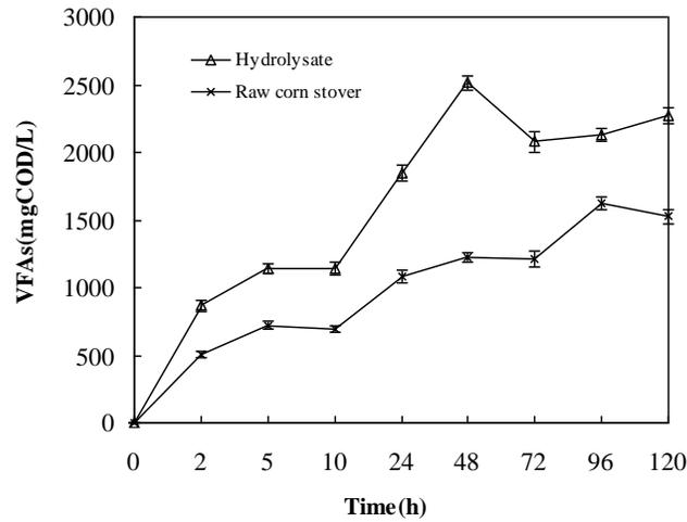
**Fig. 5.** Time-course profiles of VFA production during the anaerobic acidogenic fermentation of both hydrolysate obtained at optimum hydrolysis conditions and raw corn stover
