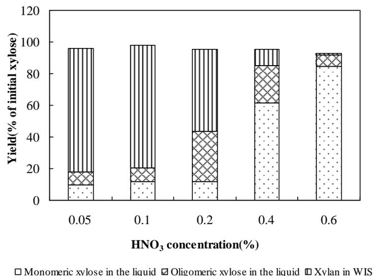
**Fig. 1.** Yields of xylose in liquids and water-insoluble solids (WISs) from the pretreatments at 150 °C for 10 min with different  $\text{HNO}_3$  concentrations
