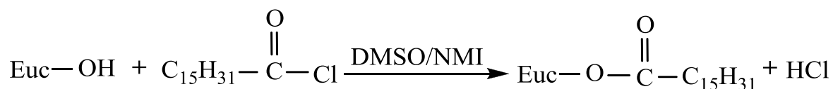
Fig. 1. Esterification of eucalyptus wood with palmitoyl chloride in DMSO/NMI solvent system without additional catalysts at room temperature
