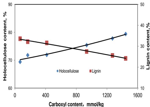
**Fig. 1.** Holocellulose and lignin content of TMP fibers with different carboxyl contents
