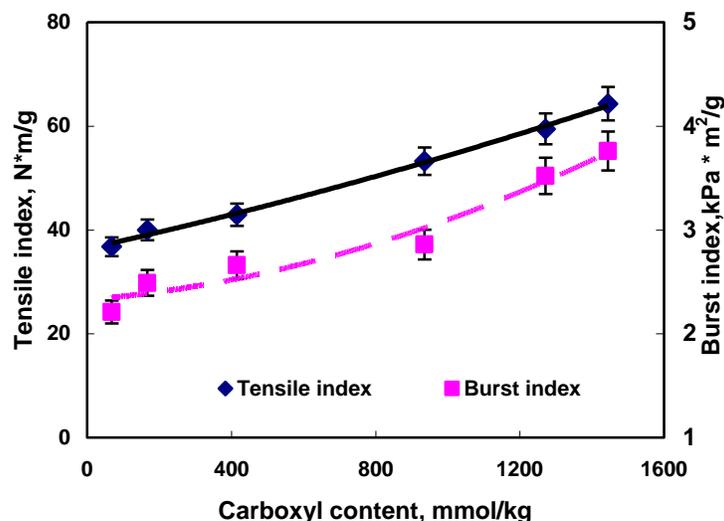
**Fig. 3.** Effect of the carboxyl content of TMP long fibers on tensile and burst strengths
