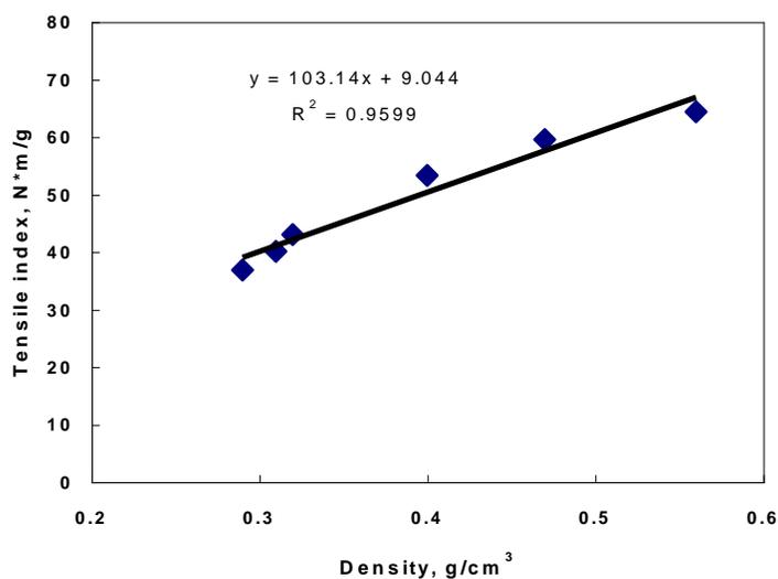
**Fig. 4.** Relationship between paper density and tensile strength for oxidized TMP long fibers
