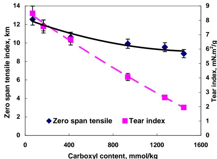
Fig. 5. Effect of carboxyl content on zero-span tensile strength and tear strength
