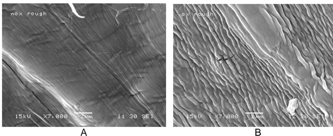
Fig. 2. Fiber surface of untreated (control) (A) and oxidized (B) TMP long fibers
