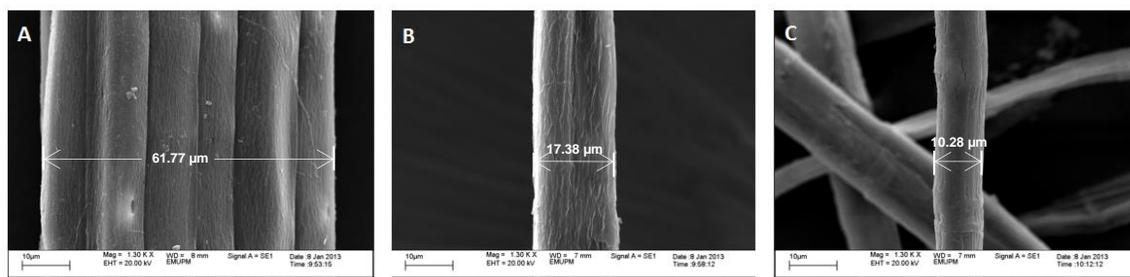
**Fig. 3.** VPSEM micrographs at 1300x magnification of A) kenaf bast fiber, B) cellulose, and C) silane-grafted cellulose
