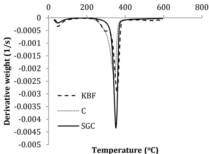
**Fig. 7.** DTG curves for kenaf bast fiber (KBF), cellulose (C), and silane-grafted cellulose (SGC)
