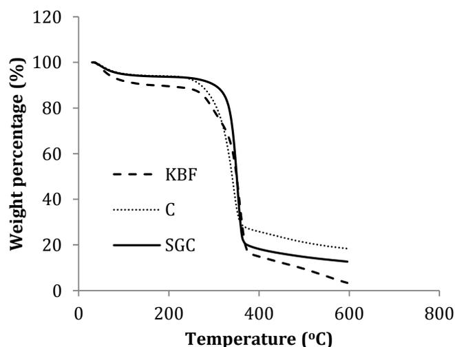
Fig. 6. TGA curves for kenaf bast fiber (KBF), cellulose (C), and silane-grafted cellulose (SGC)
