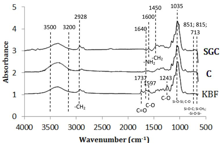
Fig. 5. FTIR spectra of KBF, C, and SGC
