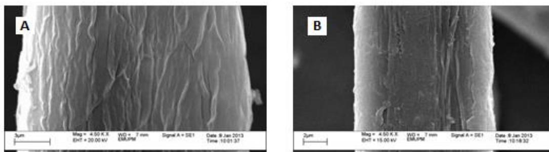
**Fig. 4.** VPSEM micrographs at 4500x magnification of A) cellulose and B) silane-grafted cellulose
