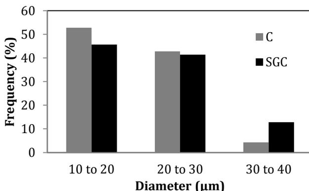
**Fig. 2.** Distribution of the diameter for composite fillers collected between 125- $\mu\text{m}$  and 250- $\mu\text{m}$  test sieves
