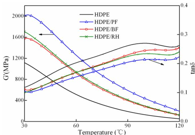
**Fig. 5.** DMA curves showing storage modulus ( $G'$ ) and loss tangent ( $\tan\delta$ ) for HDPE and composites containing natural fibers at a heating rate of 1 °C/min
