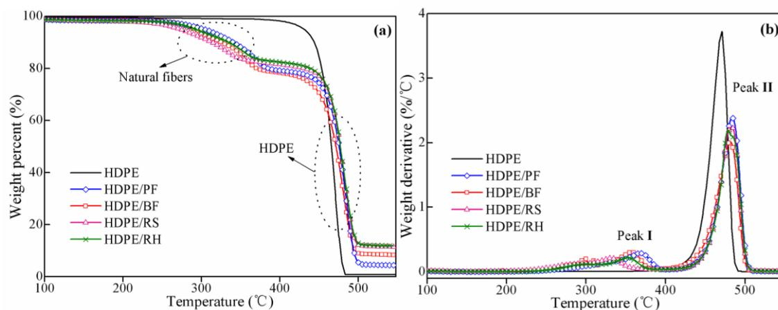
**Fig. 3.** Temperature dependence of (a) weight loss and (b) its first derivative with respect to temperature for HDPE and its composites at 10 °C/min in N<sub>2</sub>
