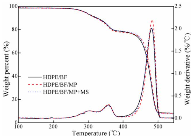
**Fig. 4.** Temperature dependence of weight loss and its first derivative with respect to temperature for the HDPE/bagasse fiber system at 10 °C/min in N<sub>2</sub>
