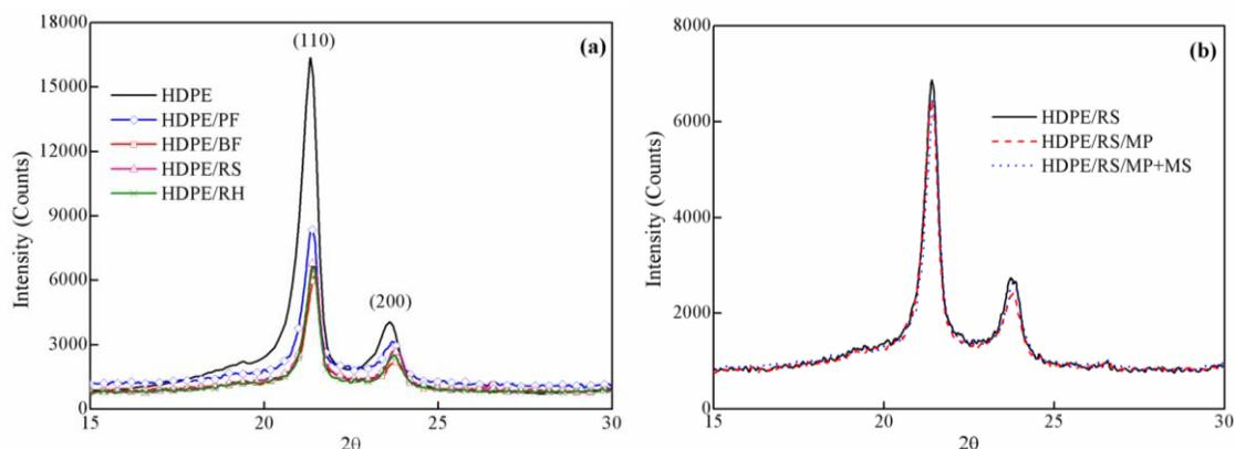
**Fig. 1.** XRD patterns for  $2\theta$  angles of 15 to  $30^\circ$  of (a) HDPE and HDPE/natural fibers composites and (b) the HDPE/rice straw system with coupling agent added
