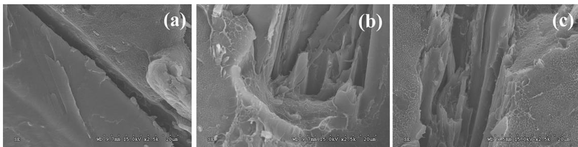
**Fig. 7.** SEM micrographs of the impact fracture surface of HDPE/bagasse fiber composites containing (a) no coupling agents; (b) 2 wt% MAPE; and (c) 2 wt% MAPE and 5 wt% MASEBS
