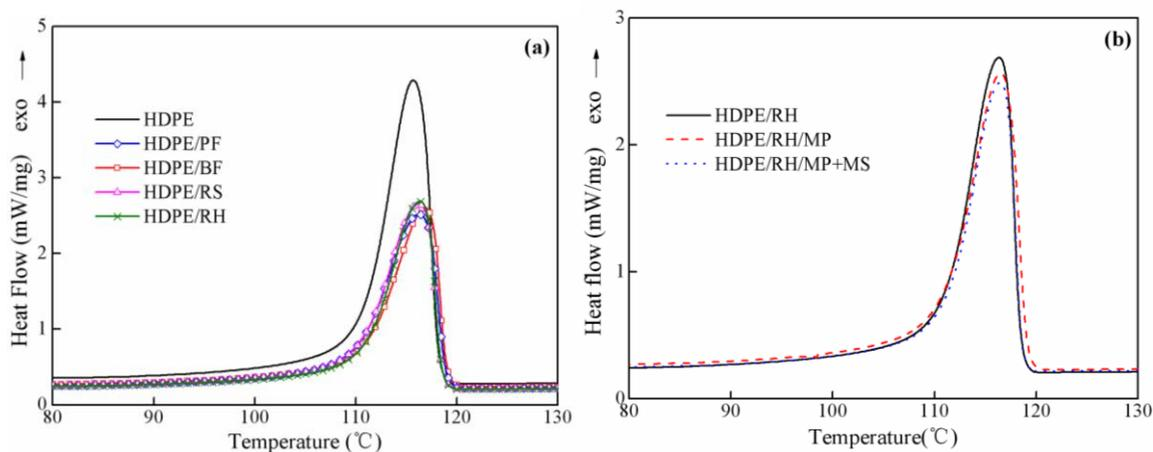
**Fig. 2.** DSC cooling curves of (a) HDPE and HDPE/natural fibers composites and (b) the HDPE/rice husk system with a coupling agent added at a cooling rate of  $10^\circ\text{C}/\text{min}$  in  $\text{N}_2$
