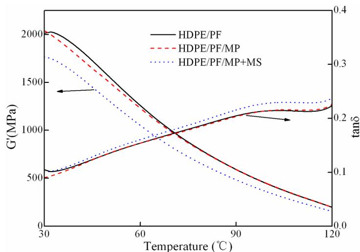
**Fig. 6.** DMA curves showing the coupling agent effect on the storage modulus ( $G'$ ) and the loss tangent ( $\tan\delta$ ) for the HDPE/pine flour system at a heating rate of 1 °C/min
