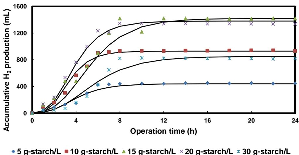
**Fig. 5.** Hourly variations of accumulative hydrogen production at various initial starch concentrations (pH: 6.5)
