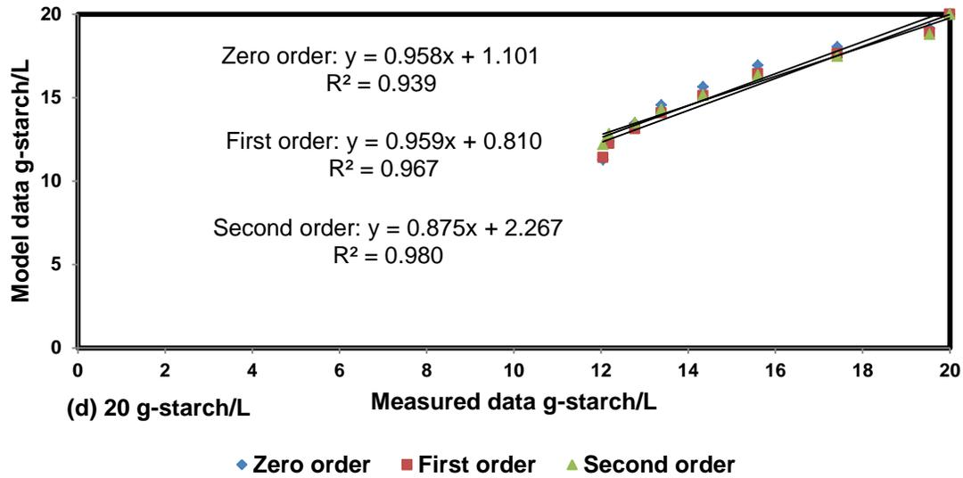
$R^2$  values between measured and modeled data for zero, 1<sup>st</sup> and 2<sup>nd</sup> orders at 20 g-starch/L
