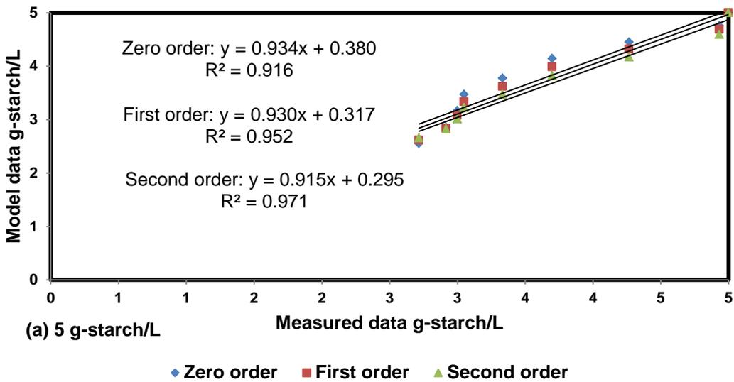
R<sup>2</sup> values between measured and modeled data for zero, 1<sup>st</sup> and 2<sup>nd</sup> orders at 5 g-starch/L
