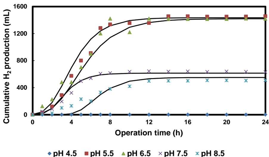
**Fig. 4.** Hourly variations of accumulative hydrogen production at various initial cultivation pH values (substrate: 15 g-starch/L)
