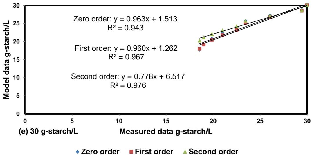
$R^2$  values between measured and modeled data for zero, 1<sup>st</sup> and 2<sup>nd</sup> orders at 30 g-starch/L
