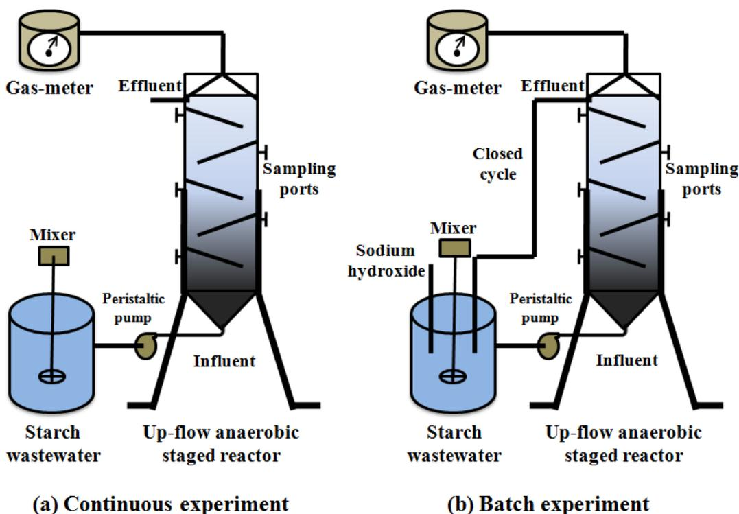
**Fig. 1.** Schematic diagram of an up-flow anaerobic staged reactor (UASR) used for (a) continuous and (b) batch experiments
