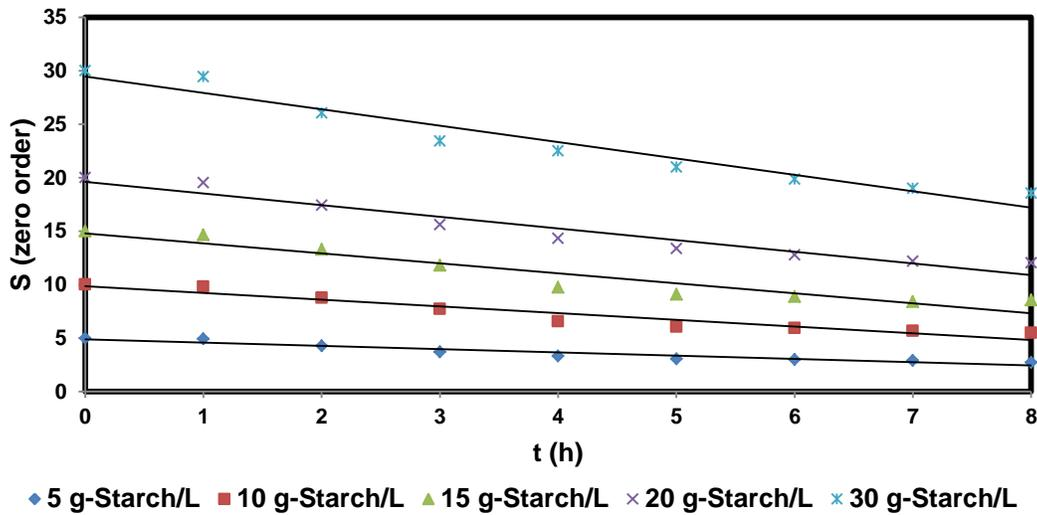
Correlation between time on x-axis and S on the y-axis for zero order at 5, 10, 15, 20, and 30 g-starch/L
