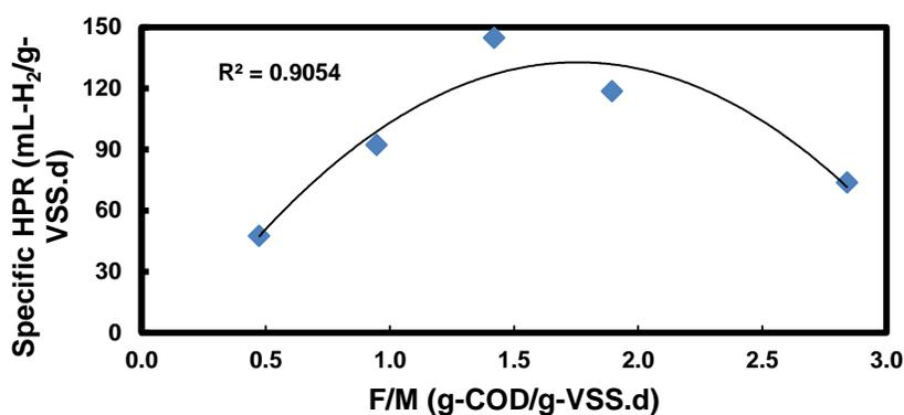
**Fig. 3.** Steady-state specific biomass hydrogen production rates from starch processing wastewater at different F/M ratios
