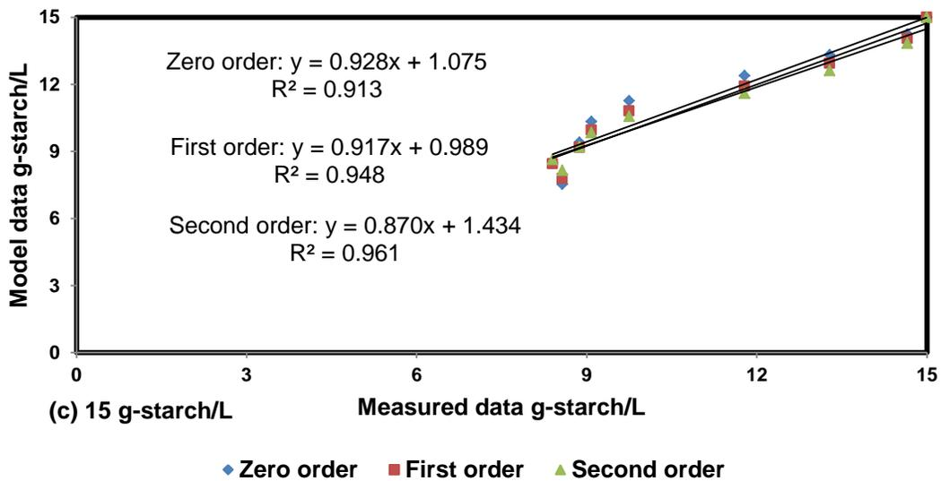
$R^2$  values between measured and modeled data for zero, 1<sup>st</sup> and 2<sup>nd</sup> orders at 15 g-starch/L
