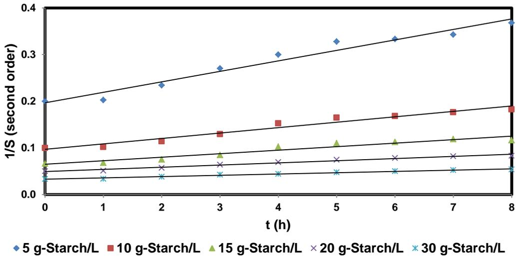
Correlation between time on x-axis and 1/S on the y-axis for second order at 5, 10, 15, 20, and 30 g-starch/L
