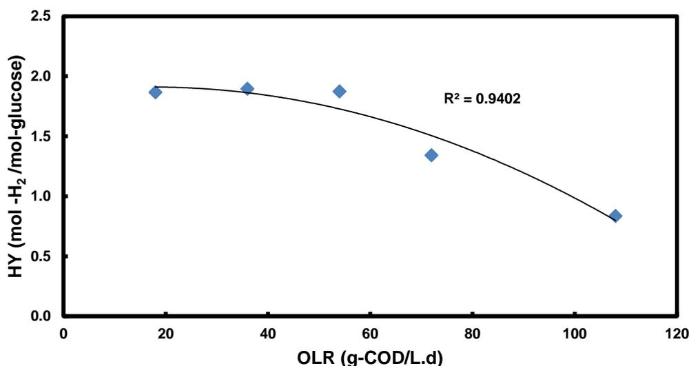
**Fig. 2.** Steady-state hydrogen yields (HY) from starch processing wastewater at different organic loading rates (OLRs)
