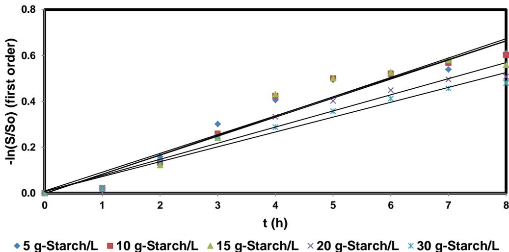
Correlation between time on x-axis and  $-\ln(S/S_0)$  on the y-axis for first order at 5, 10, 15, 20, and 30 g-starch/L
