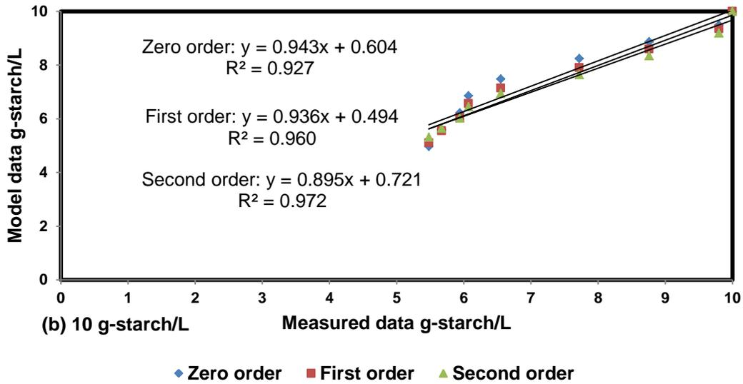
$R^2$  values between measured and modeled data for zero, 1<sup>st</sup> and 2<sup>nd</sup> orders at 10 g-starch/L
