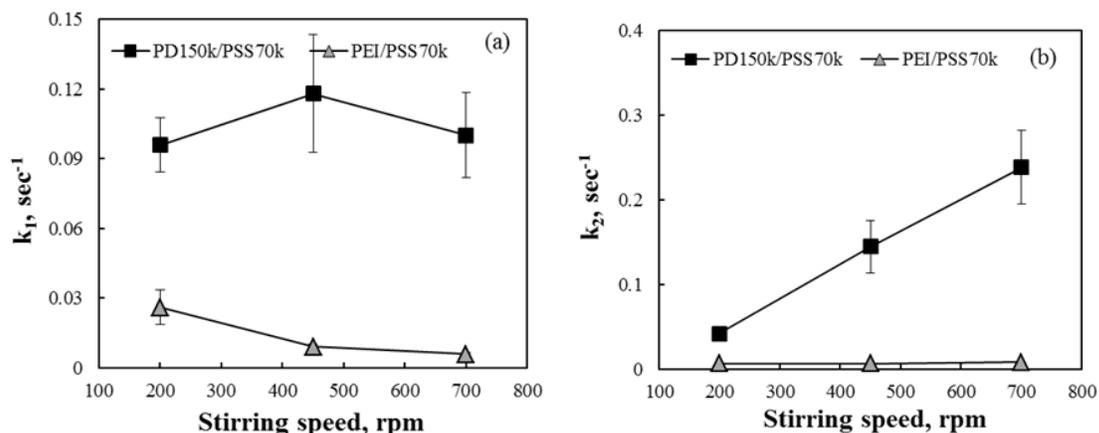
Fig. 6. Deposition kinetics (a)  $k_1$  and (b)  $k_2$  depending on shear force
