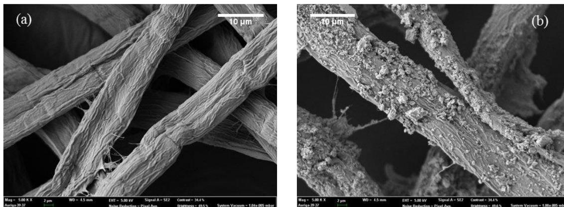
**Fig. 2.** Images of (a) fibers on which the particles are not deposited and (b) fibers on which the particles with three layers of PD<sub>150k</sub>/PSS<sub>70k</sub> are deposited at steady state
