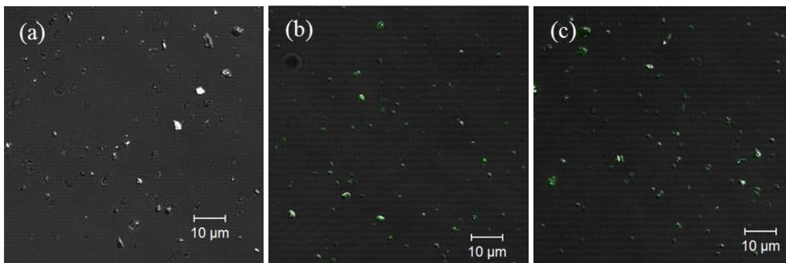
**Fig. 1.** CLSM images of (a) untreated GCC particles, (b) particles with three layers of PD<sub>150k</sub>/PSS<sub>70k</sub>, and (c) particles with three layers of PEI/ PSS<sub>70k</sub>
