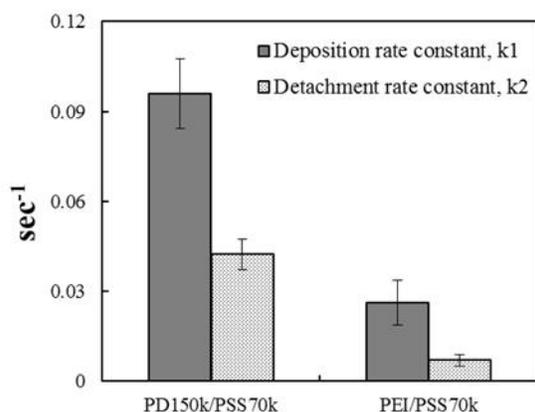
**Fig. 4.** Effect of different LbL systems on the deposition kinetic parameters
