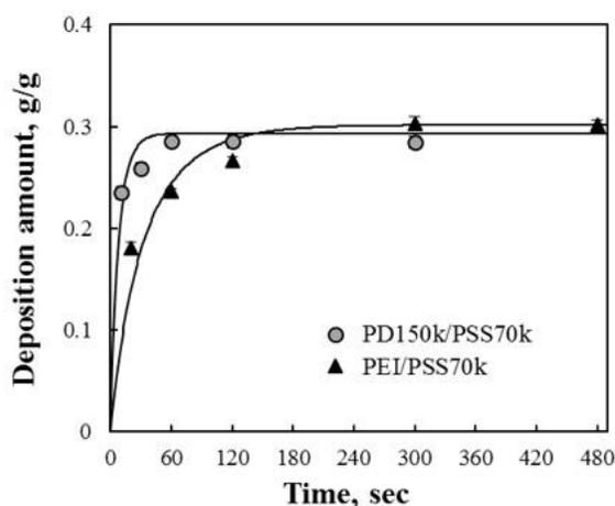
**Fig. 3.** Amount of particles with different LbL systems (3 layers) deposited on fibers as a function of time depending on polyelectrolyte types (addition amount is 0.5 g<sub>particles</sub>/g<sub>fibers</sub>). The dots represent experimental results, and the lines are theoretical results that were fit from Eq. 5 and divided by  $\Gamma_{max}$ .
