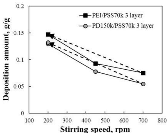
Fig. 7. Deposition amount depending on shear (addition amount is 0.2 g<sub>particles</sub>/g<sub>fibers</sub>). The dashed lines mean reducing the stirring speed to 200 rpm after pre-stirring at 700 rpm.
