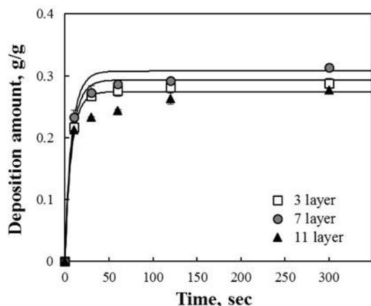
**Fig. 5.** Amount of particles with the PD<sub>450k</sub>/PSS<sub>1,000k</sub> multilayer deposited as a function of time depending on the layer number (addition amount is 0.5 g<sub>particles</sub>/g<sub>fibers</sub>). The dots are experimental results, and the lines are theoretical results that were fit from Eq. [5] and divided by  $\Gamma_{max}$ .
