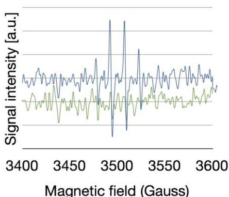
**Fig. 5.** ESR signals obtained with DMPO for ozone (in green) and ozone and maleic acid (in blue)
