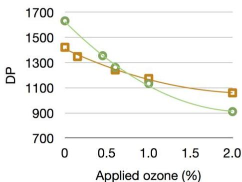
**Fig. 1.**  $DP_v$  versus ozone charge for HexA- and lignin-free pulp (squares) in comparison with the behavior of the oxygen-delignified pulp (circles)
