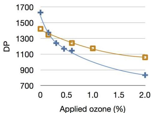
**Fig. 2.**  $DP_v$  of a HexA- and lignin-free pulp (squares) and of a lignin-free pulp (crosses) at various ozone charges
