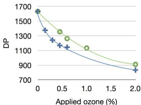
**Fig. 3.**  $DP_v$  of a lignin-free pulp (crosses) and a Kraft+O pulp (circles) at various ozone charges
