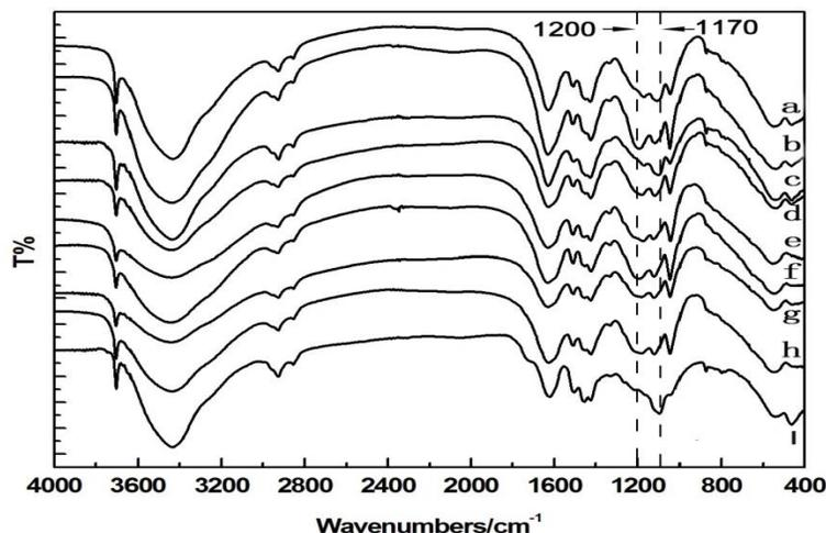
**Fig. 2.** FT-IR spectra of stratified alkaline precipitates and acid-insoluble lignin. (a-d) upper layer of precipitate at pH 10,11,12,13, respectively; (e-h) lower layer of precipitate at pH 10,11,12,13, respectively; (i) acid-insoluble lignin
