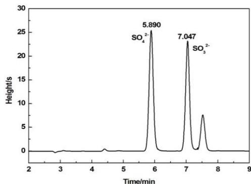
**Fig. 3.** Ion chromatogram of  $\text{SO}_4^{2-}$  and  $\text{SO}_3^{2-}$
