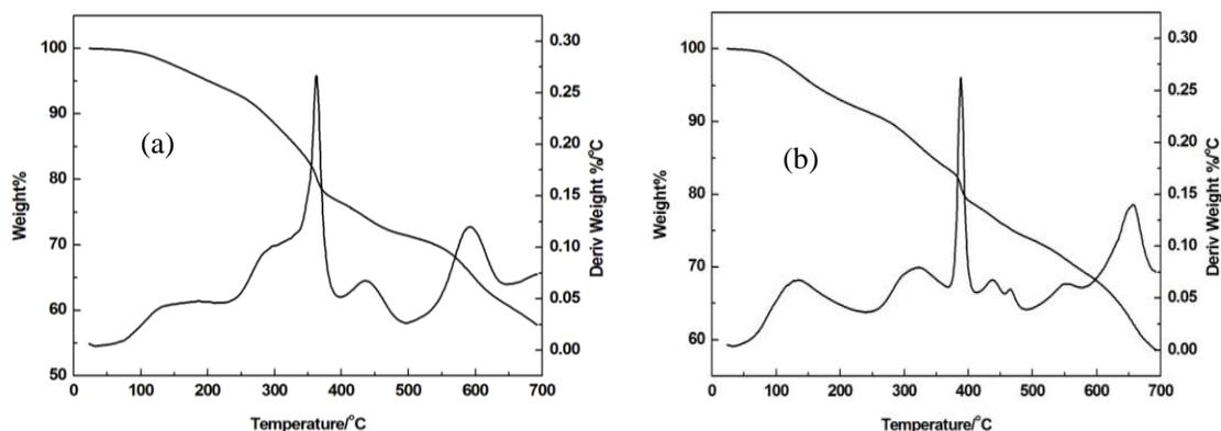
**Fig. 5.** TGA and DTA of stratified alkaline precipitation: (a) upper layer of precipitate; (b) lower layer of precipitate
