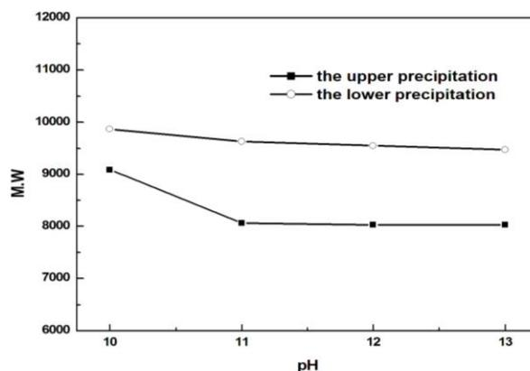
Fig. 6. Relative molecular weight of stratified alkaline precipitation
