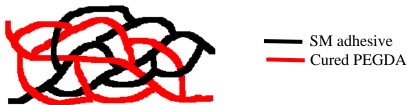
Fig. 7. Interpenetrating polymer networks (IPNs) of cured PEGDA and SM adhesive
