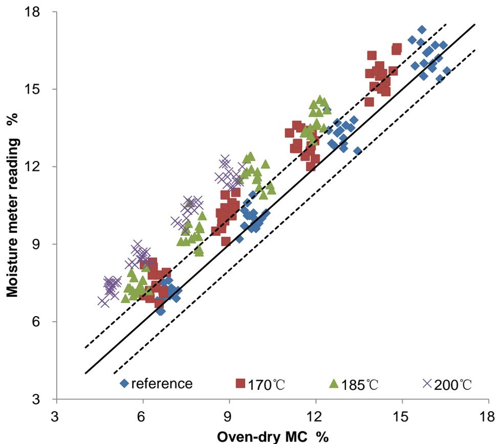
**Fig. 3.** Moisture meter reading versus oven-dry MC for the reference specimens and heat-treated wood of Mongolian pine
