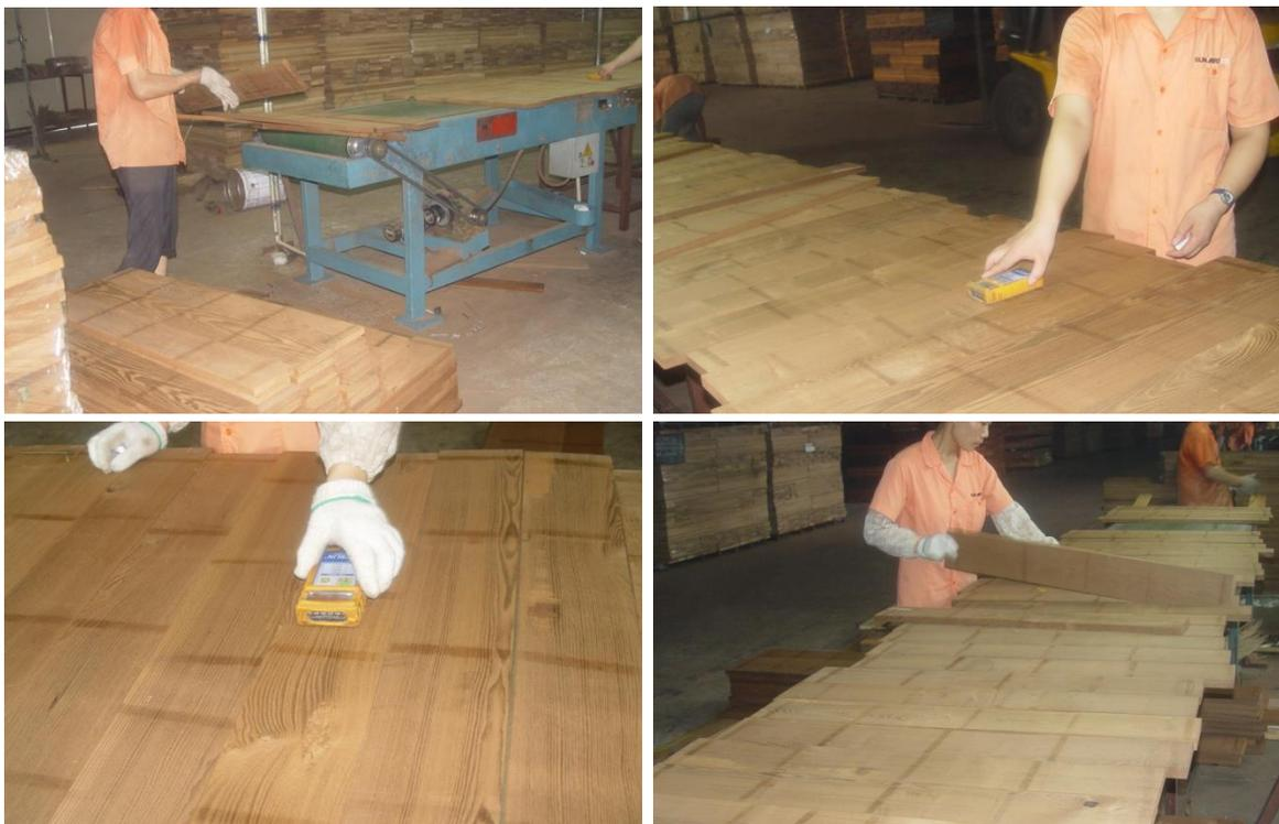
**Fig. 1.** A special production line for checking the drying quality and MC of kiln-dried planks
