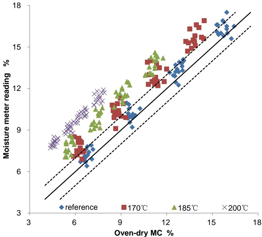
**Fig. 2.** Moisture meter reading *versus* oven-dry MC for the reference specimens and heat-treated wood of Manchurian ash
