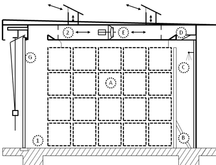
**Fig. 1.** Sectional drawing of a kiln with timber packages (A), stand (B), water spraying (C), damper register (D), and fan (E). Specimens were taken from the bottom (1) and from the intermediate ceiling (2).
