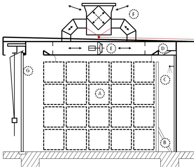
**Fig. 3.** Sectional drawing of a kiln chamber with timber packages (A), stand (B), water spraying (C), damper register (D), fan (E), and heat exchange device where condensate is ideally recovered (F); see red line.
