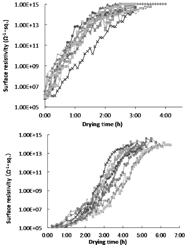
**Fig. 5.** Changes in electrical resistivity of the surface of *Cryptomeria japonica* heartwood (upper: twelve samples of red heartwood, lower: ten samples of black heartwood); the sq. stands for square.
