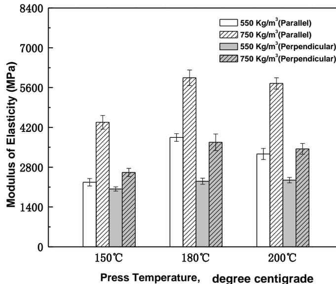
Fig. 3. Effects of press temperature and density on MOE of CBP (laminated with MDF)
