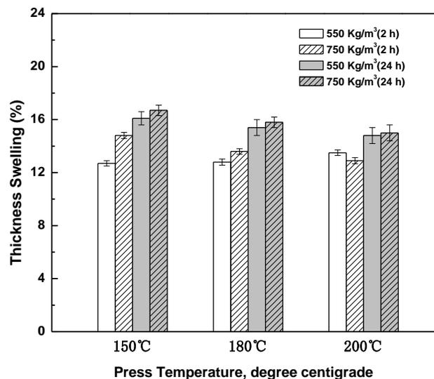
**Fig. 4.** Effects of press temperature and density on TS of CBP
