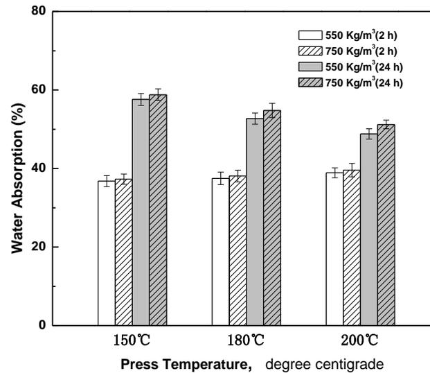
Fig. 5. Effects of press temperature and density on WA of CBP
