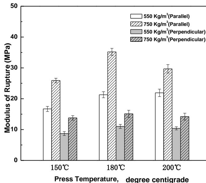
**Fig. 2.** Effects of press temperature and density on MOR of CBP (laminated with MDF)
