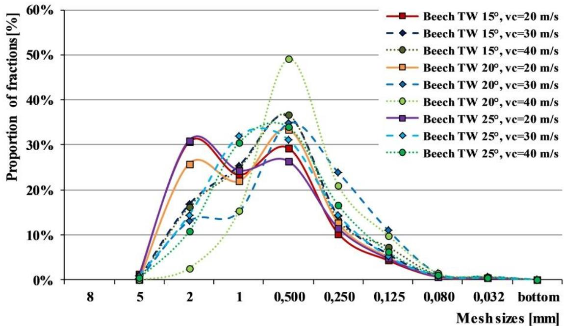
Fig. 9. Effect of cutting speeds on splinter size distribution of TW beech at feed speed  $v_f = 8$  m/min
