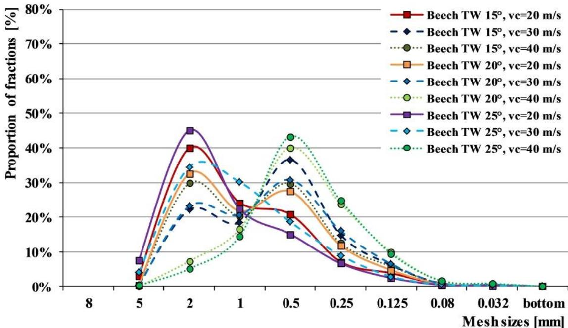
Fig. 11. Effect of cutting speeds on splinter size distribution of TW beech at feed speed  $v_f = 11$  m/min
