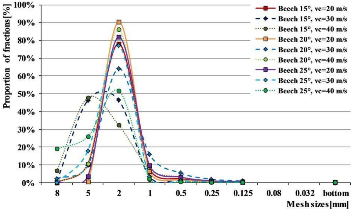
Fig. 6. Effect of cutting speeds on splinter size distribution of natural beech at feed speed  $v_f = 4$  m/min
