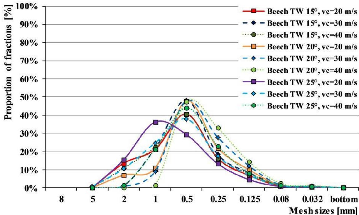
Fig. 7. Effect of cutting speed on splinter size distribution of TW beech at feed speed  $v_f = 4$  m/min
