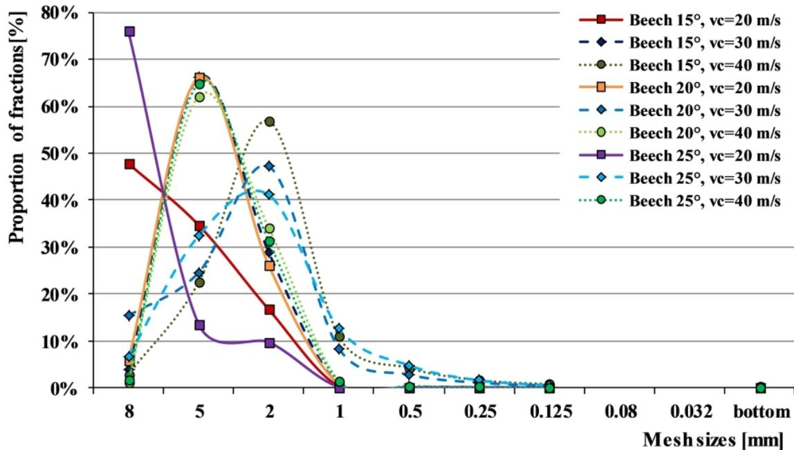
Fig. 10. Effect of cutting speeds on splinter size distribution of natural beech at feed speed  $v_f = 11$  m/min
