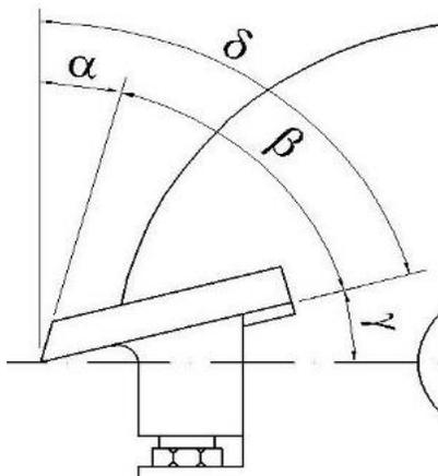
**Fig. 4.** The angles of the cutting blades fitted in cutter head (Prokeš 1982)
