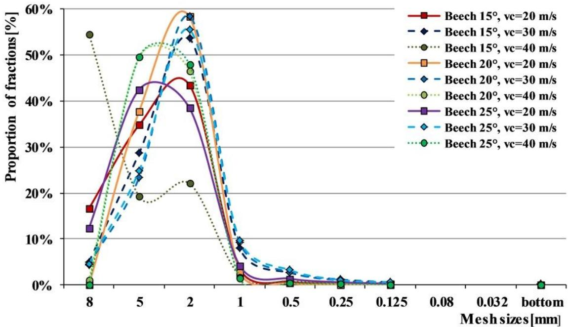
Fig. 8. Effect of cutting speed on splinter size distribution of natural beech at feed speed  $v_f = 8$  m/min
