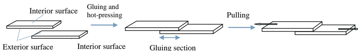
Fig. 1. Method of measurement of shear strength of specimens glued with UF, PF, and MDI
