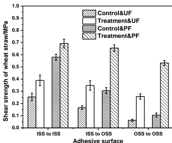
**Fig. 4.** The shear strength of the untreated and plasma-treated wheat straw on different adhesive surfaces of UF and PF
