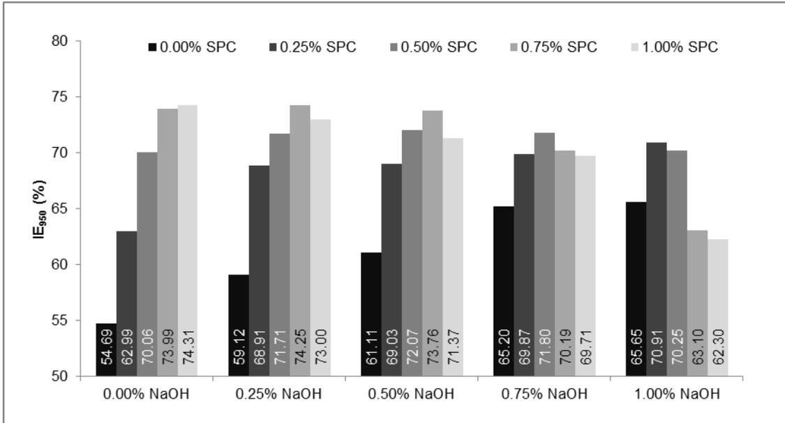
Fig. 9. Effects of S<sub>p</sub>C charges on ink elimination ratio of deinked pulps
