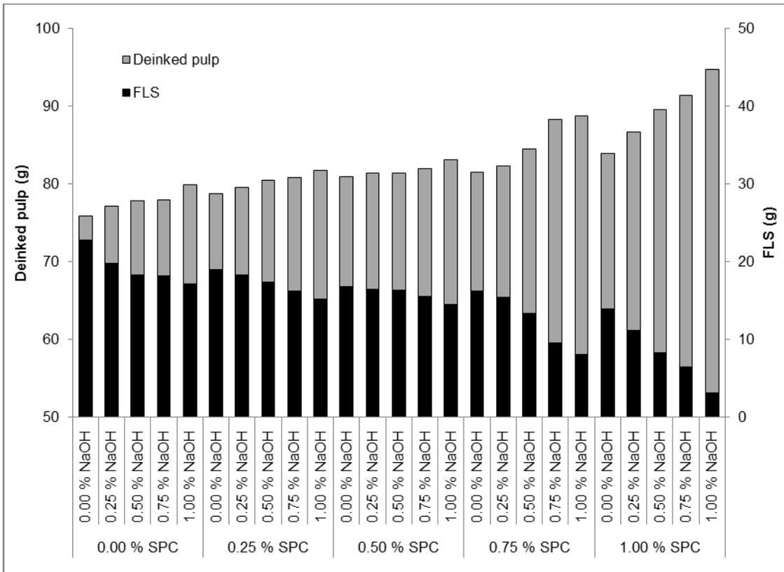
Fig. 10. Effects of S<sub>p</sub>C charges on yield parameters of pulps
